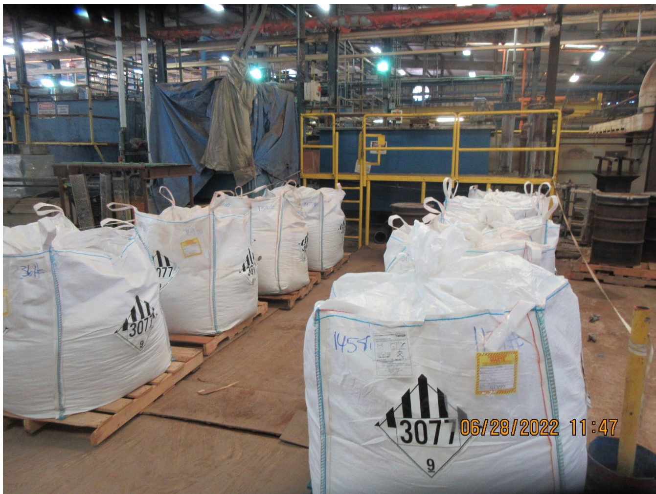
Photo 10 – Cubic Yard Bags of F006 Hazardous Waste Sludge in Overflow Area
