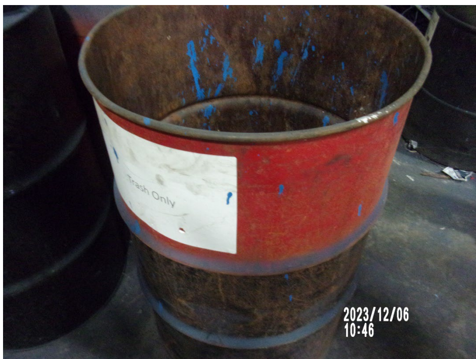
Photograph 9: Collection Container for Punctured Aerosol Cans Inappropriately labeled as "Trash Only".
