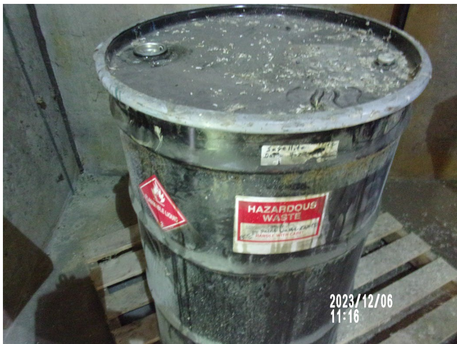
Photograph 15: A new bung hole cap has been inserted. Container is not closed.
