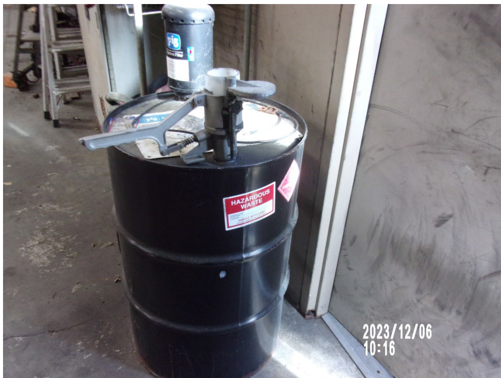
Photograph 2: Open Satellite Accumulation Container.
