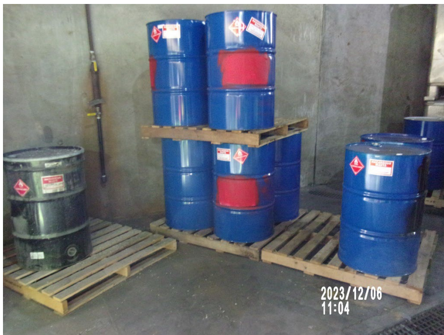
Photograph 13: 55-Gallon Hazardous Waste Containers in the Central Accumulation Area (CAA).
