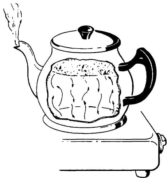
Figure 3-8. Heat Transfer by Convection
