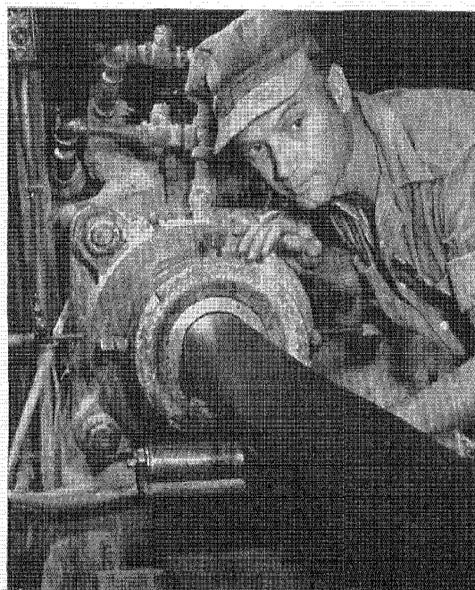
Lubricants added to raw stock during milling facilitate extrusion of inner tubes.
