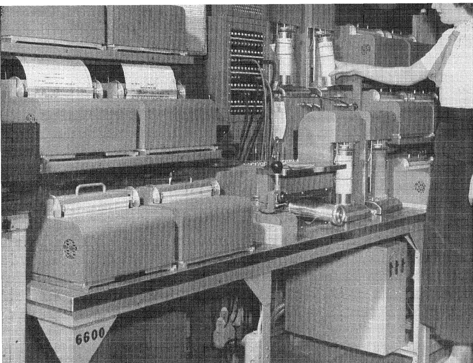
Western Union operator inserts telegram in facsimile equipment for transmission. At left, telegrams are received on recording paper.
