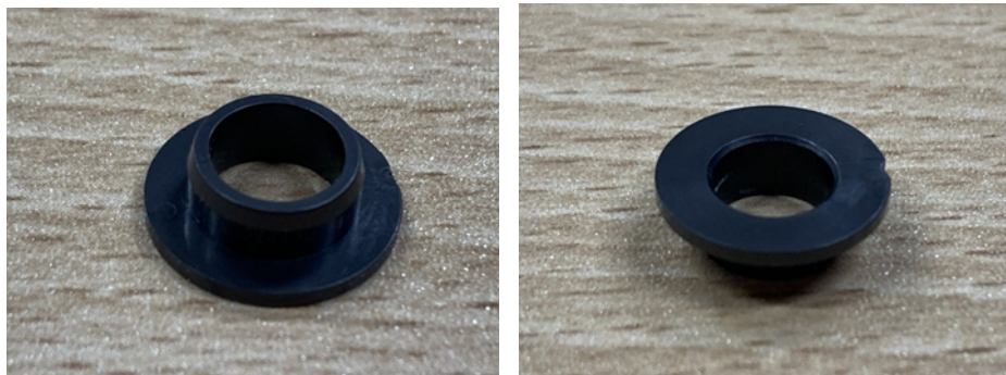
Figure 10 The bobbin pipe in the mechanism that locks the IP cassette that stores IP in CR
