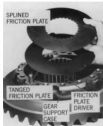
Removing Tanged and Splined Friction Plates
