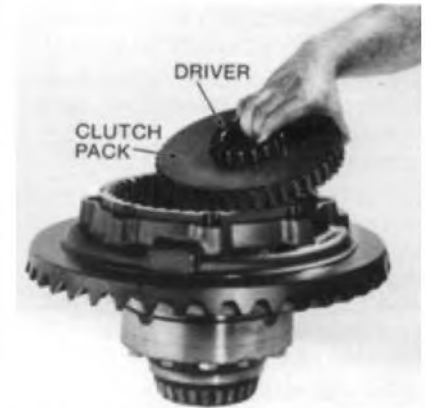
installing Clutch Pack and Driver Assembly (Permanent CTD Only)
