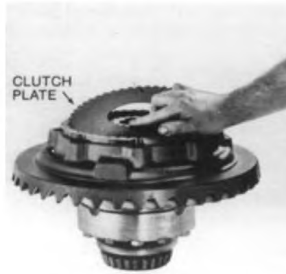
Installing Clutch Plates Individually (Permanent CTD Only)
