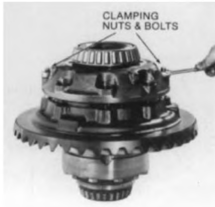
Removing Clamping Nuts and Bolts
