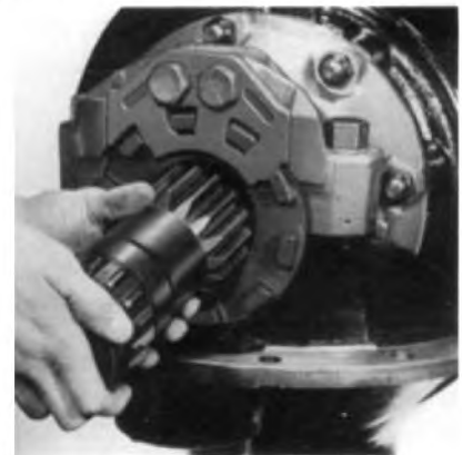
Removing Sliding Clutch
