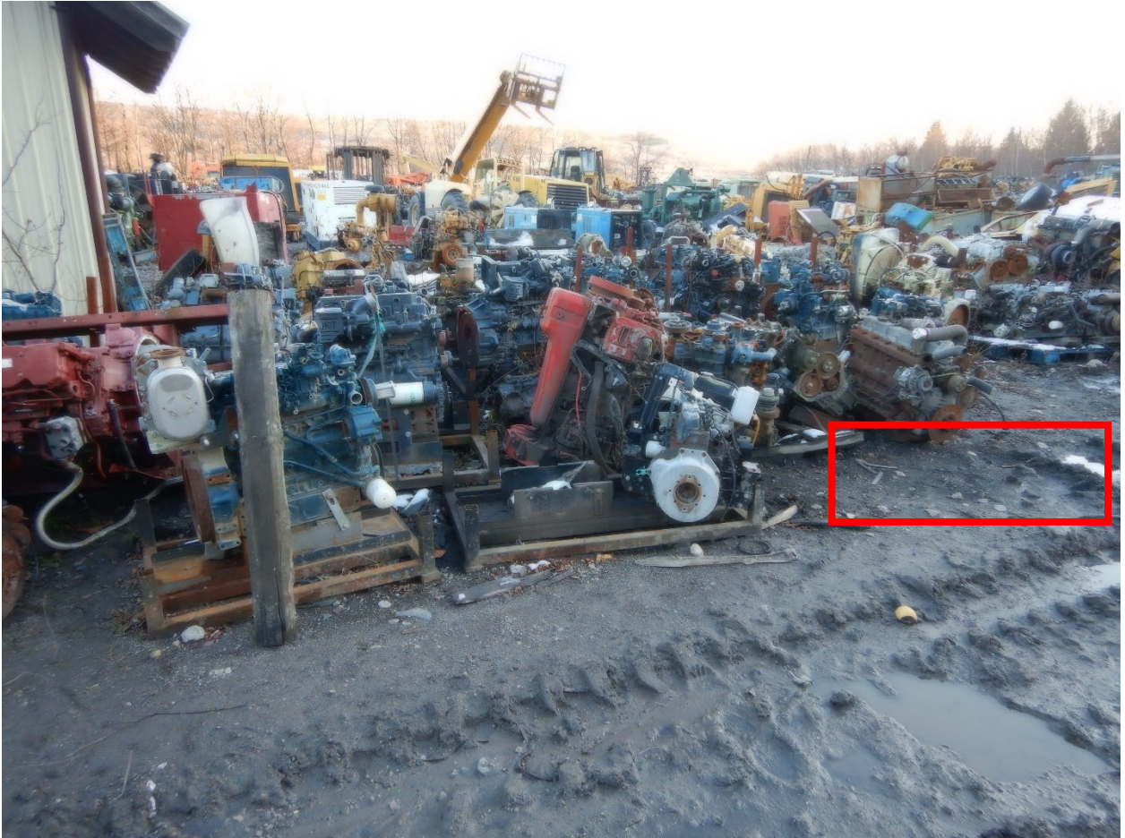
DSCN4067 Pumps and engine parts in facility yard – note dark staining surrounding parts (red box)
