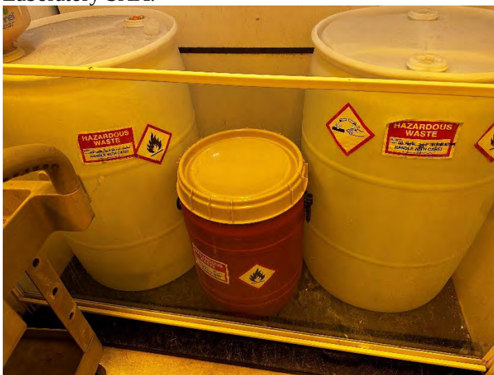
Photograph 4: 2-55-gallon drums of laboratory waste mixed with spent solvents and a hazardous waste container of dissolution HCL in the Quality Control Laboratory SAA.
