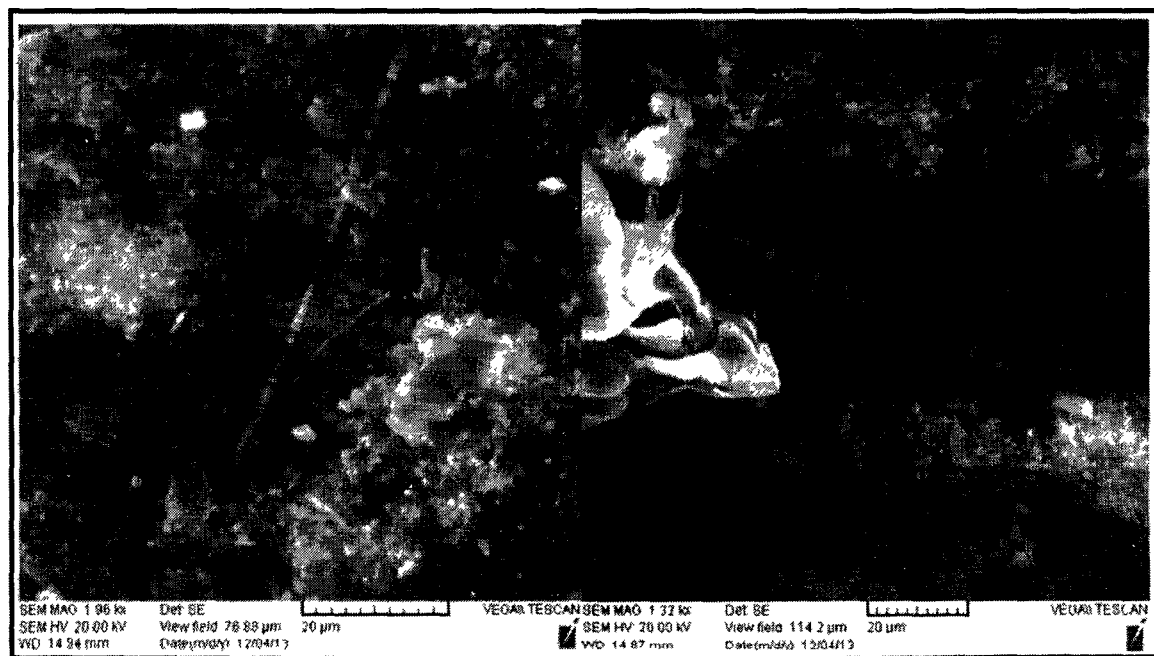
Figure 11 These are asbestos bodies from the patients lung tissue taken by SEM. It is possible to see in the one to the left that the fiber is almost completely covered by the iron protein coating. This is compared to the one at the right which appears to have much more fiber exposed. However, upon EDS testing, it was determined that in both cases, these were anthophyllite fibers and they were both entirely coated, although much thicker in some areas as opposed to others.
