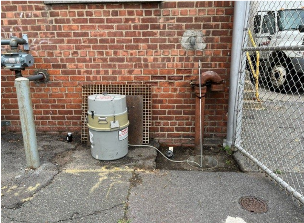
Photo #1. An ISCO automatic composite sampler was set-up at the monitoring location.
