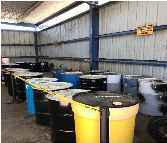
Photo-9 CAA-Inadequate Aisle Space
