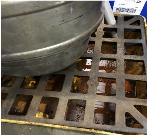
Photo-12 CAA- Used Oil in Secondary Containment
