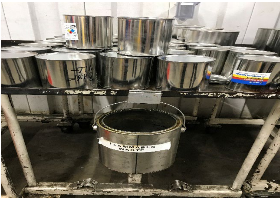
Photo-4 Tool Room, Open SAA Container
