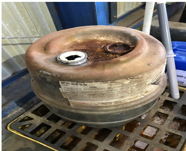
Photo-8 CAA Open D002 Waste Container, D002 Waste in Secondary Containment
