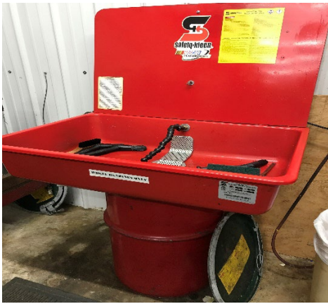
Photo-3 Parts Washer, Tool Room
