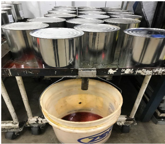
Photo-6 Tool Room, Open Container with waste accumulation
