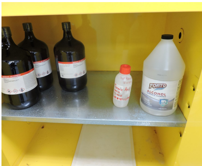
Picture 15 - UPR CHEMICAL ENGINEERING- At the Lab IQ-103 A there were three 4-L ambar containers with Methanol stored next to one (1) 500-ml bottle with Formic Acid and next to one (1) 1-gallon plastic bottle container Ethy Alcohol 70% without following any safety protocols or compatibility characteristic.
