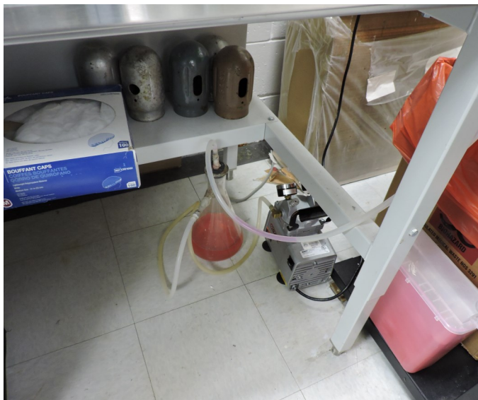
Picture 1 - UPR CHEMICAL ENGINEERING- At the Lab IQ-101 K there was one (1) 1-liter Erlenmeyer Flask with a “Biohazard Waste,” unlabeled and without hazardous waste determination if it is managed as an lab waste, the content and the container must be labeled and date as “Unwanted Material.”
