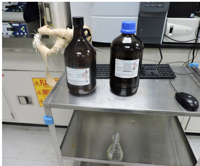
Picture 6 - UPR CHEMICAL ENGINEERING- At the Lab IQ-101 J there were four 4-L containers stored in trays containing THF and 1,4-Dioxane dated as July 16, 2019, and March 3, 2020, not in use and abandoned and not managed as “Unwanted Material,” without a hazardous waste determination.
