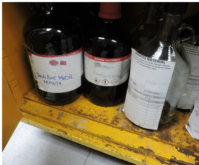
Picture 8 - UPR CHEMICAL ENGINEERING— At the Lab IQ-101 HI there were six (6) 4-liter ambar containers stored inside a cabinet area only two were labeled as “Unwanted Materials” and one with its accumulation start date of March 3, 26, 2019 which exceeded over six months of the LMP.
