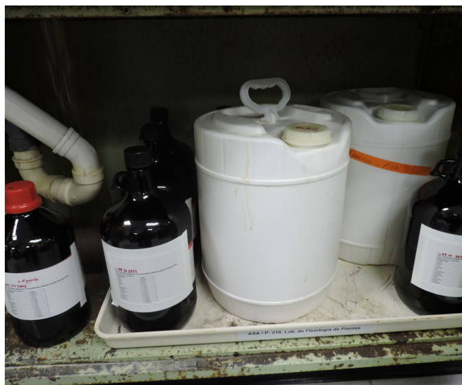
Picture 10 - UPR CHEMICAL ENGINEERING- At the Lab IQ-101 HI there were four (4) 4-L containers stored inside a cabinet sink not labeled as “Unwanted Materials,” and dated as of August 23, 2022, March 1, 2021, February 24, 2023, and other non-dated which exceeded over six months of the LMP collection protocols.
