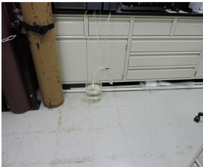
Picture 7 - UPR CHEMICAL ENGINEERING- At the Lab IQ-101 J there was one (1) 4-liter glass container with a spent mobile phase connected to a HPLC not in use since November 2022, unlabeled and without hazardous waste determination if it managed as an “Unwanted Material.”
