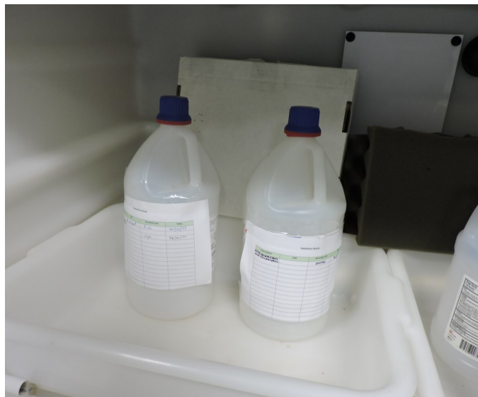
Picture 14 - UPR CHEMICAL ENGINEERING- At the Lab IQ-101 O there were two (2) 4-liter plastic containers with a spent petroleum ether and terpolymer labelled as “Unwanted Materials,” and dated with their accumulation start dates of May 15, 2022, which exceeded over six months of the LMP collection protocols.
