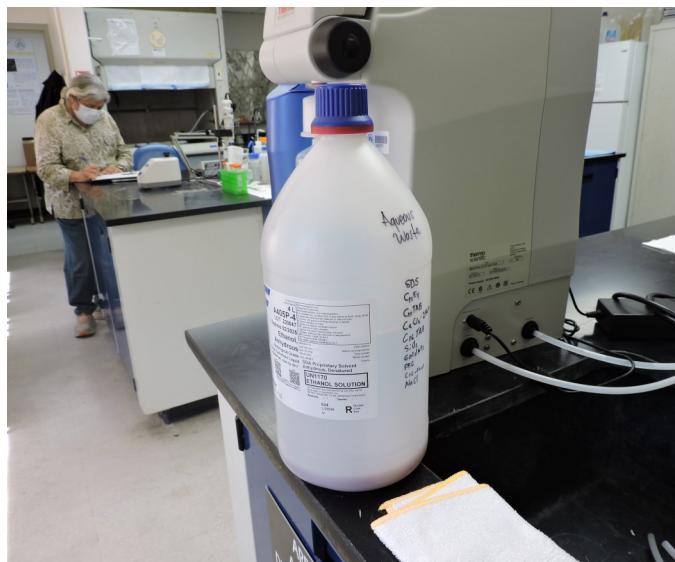
Picture 16 - UPR CHEMICAL ENGINEERING— At the Lab IQ-102 A there was one (1) 2-gallon plastic container with a spent Ethanol aqueous waste no labeled as “Unwanted Materials,” nor dated with its accumulation start date.
