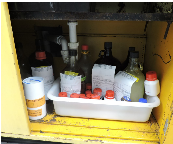
Picture 9 - UPR CHEMICAL ENGINEERING- At the Lab IQ-101 HI there were six (6) 4-liter ambar and glass containers stored inside a cabinet sink area only four were labeled as “Unwanted Materials” and with their accumulation start dates. However, three (3) were not labeled as “Universal Wastes,” nor dated .
