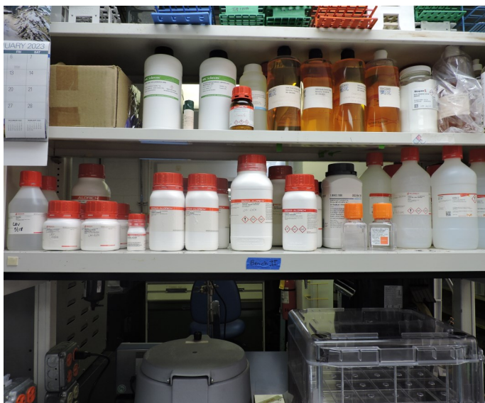
Picture 17 - UPR CHEMICAL ENGINEERING- At the Lab IQ-102 A it was observed the storage of chemical reagents at laboratory cabinets was conducted without following any safety protocols or compatibility characteristics (Flammable, Corrosives and Toxics – NaOH, Hydrochloric Methylcellulose, KCl) of the reagents.
