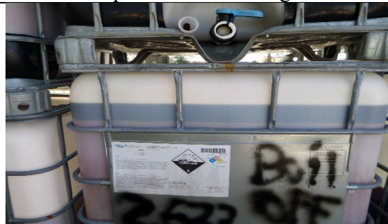
Photo-22 Unlabeled Corrosive Waste (D002)
