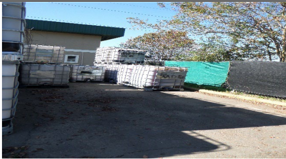
Photo-2 Process Water Tote Storage, Unlabeled totes with no hazard indication
