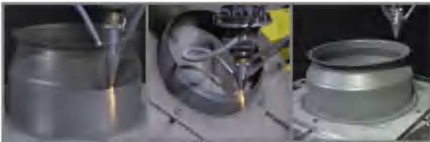
Fig. 9.13 LMD processed helicopter engine combustion chamber
