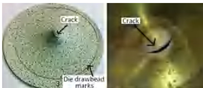
Fig. 24.3 Examples of broken punch test specimens. The broken specimen is coated in paint for DIC (left) and the revealed crack after the speckled coating is removed from the specimen surface (right)
