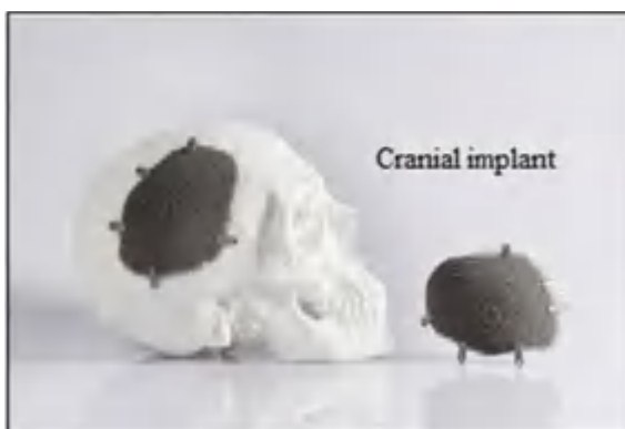
Fig. 9.15 Titanium lattice cranial implant manufactured using additive manufacturing
