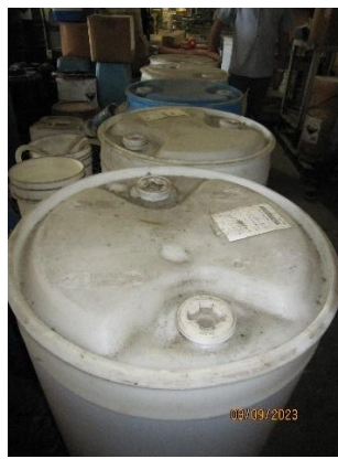
Photo #30 – Seven 55-gallon containers of non-treated plating waste.
