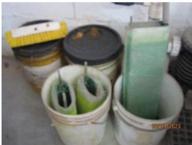
Photo #33 – Open containers of spent chrome filter sleeves.
