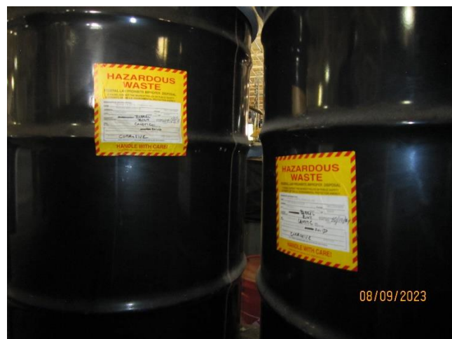
Photo #12 – Two 55-gallon containers of “Caustic Solid Corrosive” waste.
