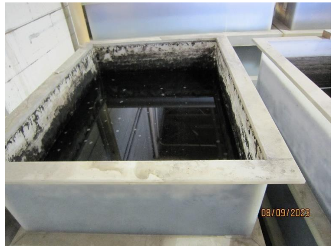
Photo #20 – Plating waste stored in the poly tank.
