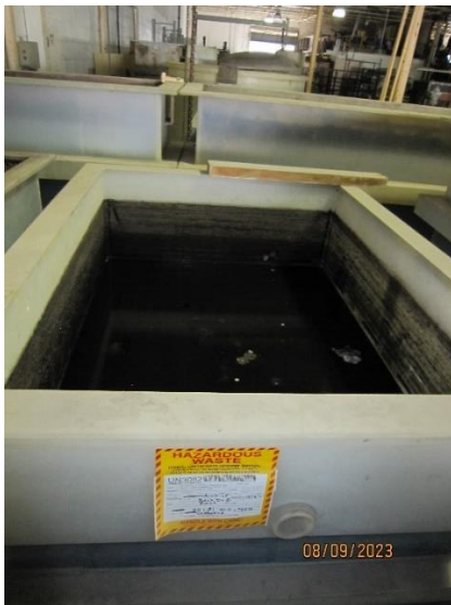
Photo #19 – Plating waste stored in the poly tank.
