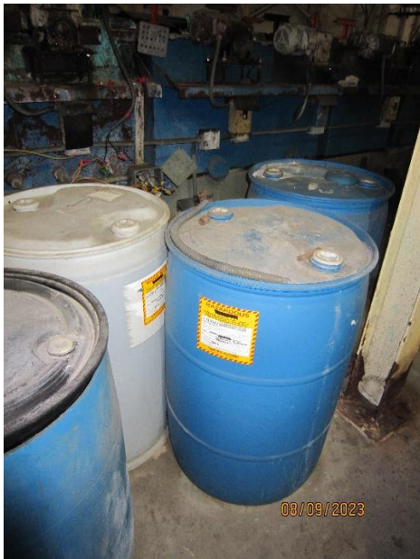
Photo #5 – 55-gallon containers of cadmium plating solution in storage for reuse.
