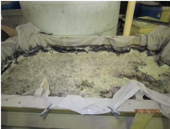
Photo #17 – Plating waste stored in the poly tank.
