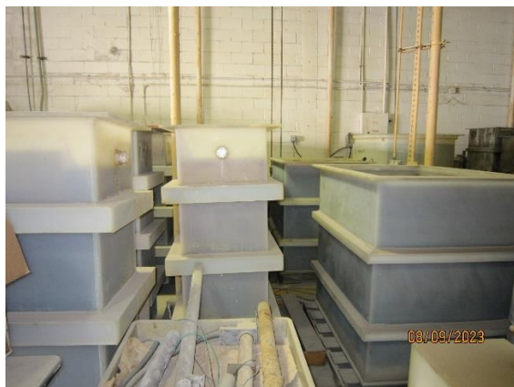
Photo #15 – Plating waste stored in the poly tanks.
