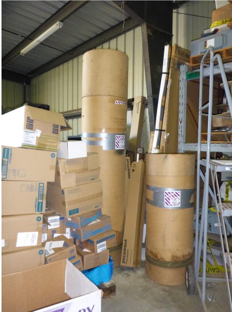
Photo 21: One 8-foot cardboard cylinder, one 4-foot cardboard cylinder, two 4-foot cardboard boxes and one open, square cardboard box in the foreground, which all appeared to contain universal waste lamps. The cylinders were each labeled as universal waste lamps and dated 10/07/2020. None of the cardboard boxes were labeled or dated. Additional 8-foot cardboard boxes observed behind these containers. Those additional boxes appeared to contain either new or universal waste lamps.
