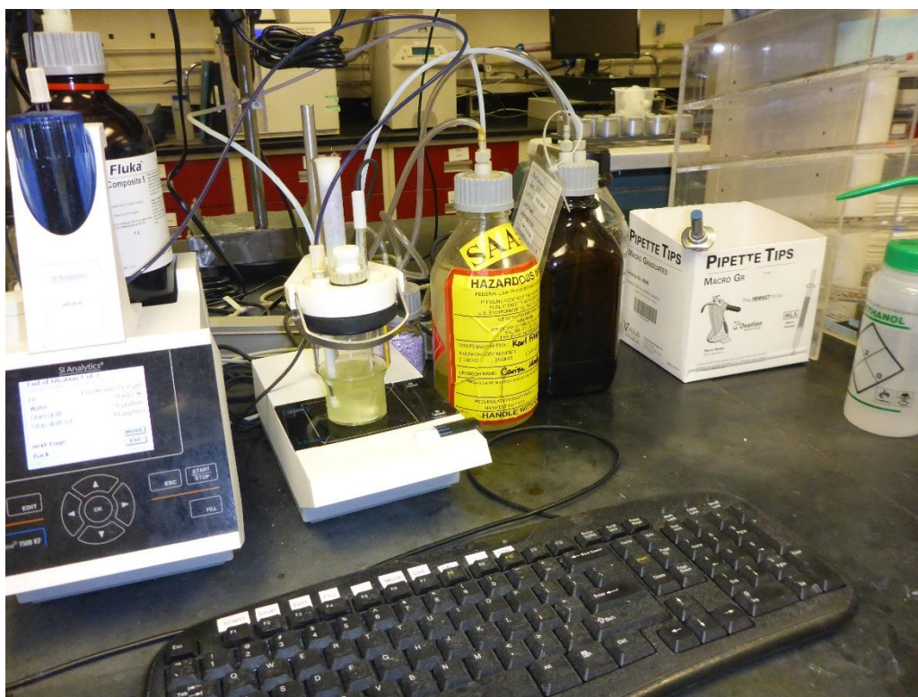
Photo 11: One one-liter jar at SAA #10, which is used to accumulate hazardous waste flammable liquids that are generated by the Karl Fisher unit. The jar was labeled as SAA #11 and hazardous waste and identified with a flammable liquid DOT hazard placard.
