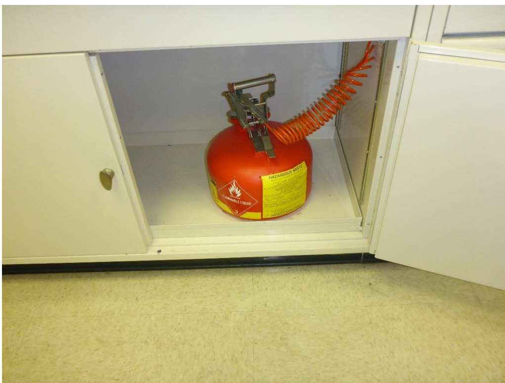
Photo 9: One one-gallon flammable can at SAA #8, which is used to accumulate hazardous waste flammable liquids that are generated in the PD laboratory. The can was labeled hazardous waste and identified with a flammable liquid DOT hazard placard.
