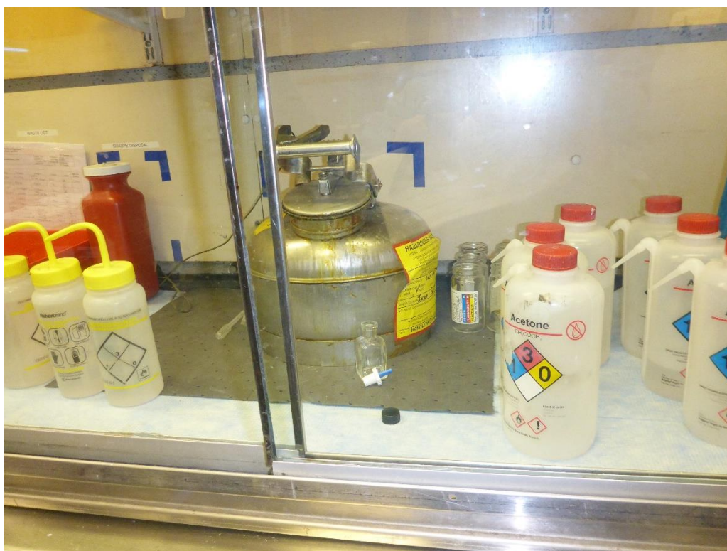
Photo 10: One two-gallon container at SAA #9, which is used to accumulate hazardous waste flammable liquids that are generated by sample analysis in the laboratory. The container was labeled as SAA #9 and hazardous waste and identified with a flammable liquid DOT hazard placard.
