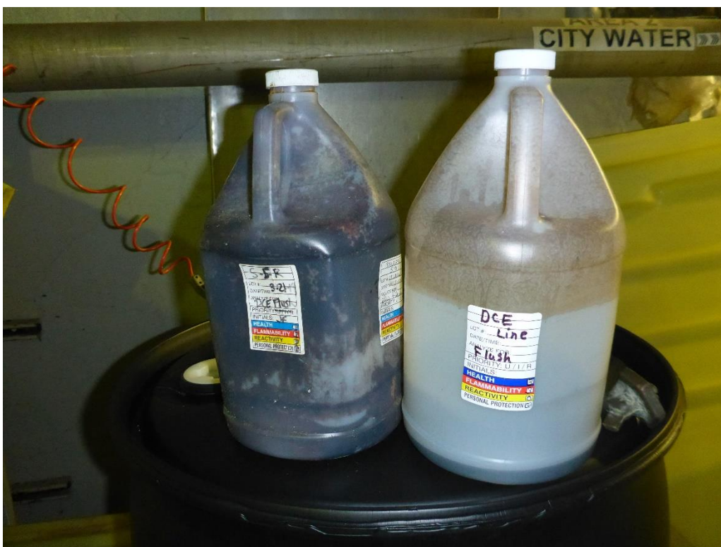
Photo 6: Two one-gallon jugs inside the locked, plastic clam-shell secondary containment unit at SAA #4. The jugs were each labeled DCE Line Flush and identified with a Hazcom label. One jug was dated 03/21/2019.
