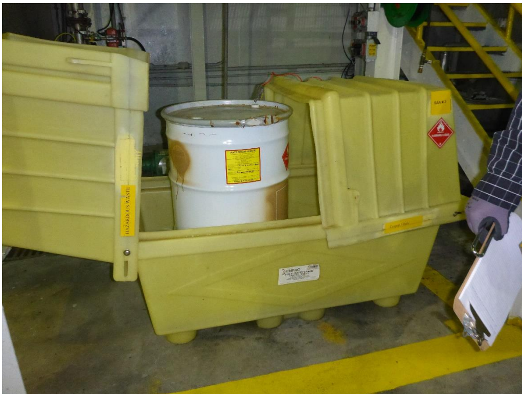
Photo 2: One 55-gallon drum inside a locked, plastic clam-shell secondary containment unit at SAA #2, which is used to accumulate hazardous waste filters that are generated by the Celquat process. The clam-shell was identified as SAA #2, labeled hazardous waste and marked with a flammable liquid DOT hazard placard. The drum was labeled hazardous waste flammable liquid and identified with a flammable liquid DOT hazard placard.
