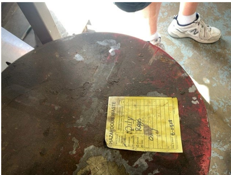
Photo 37 – Oily rags container observed in the IFAS maintenance shop missing a toxic indication of hazard.
