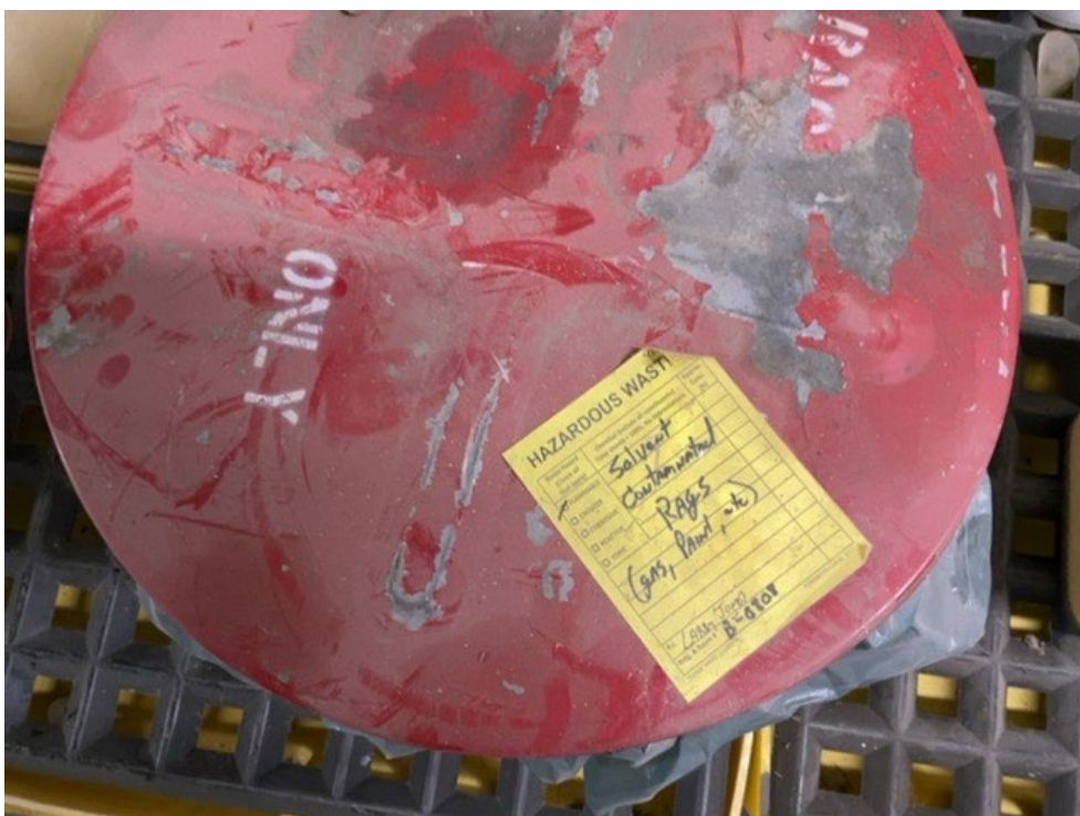
Photo 34 – Container of solvent contaminated rags missing the toxic indication of hazards.
