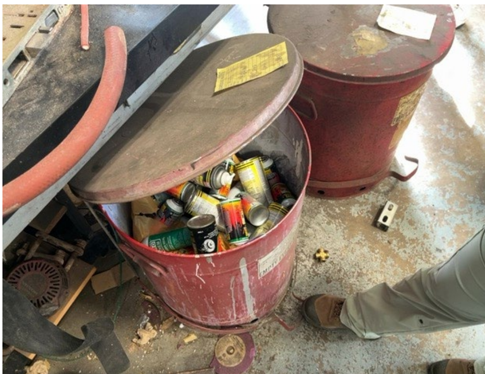
Photo 36 – Aerosol waste container observed outside of the IFAS maintenance shop. This container was missing a toxic indication of hazard.
