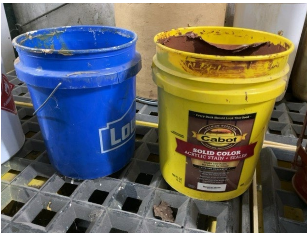
Photo 33 – Open RCRA-empty containers in the IFAS paint shop SAA.
