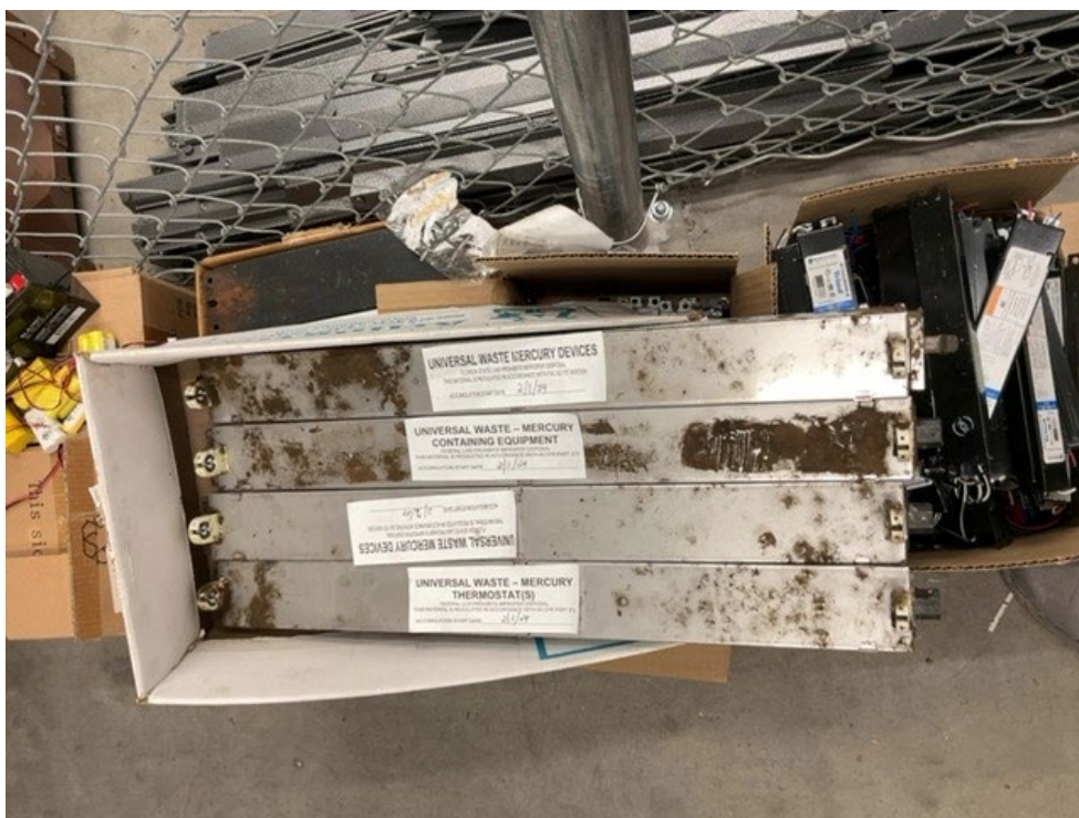
Photo 31 – Mercury equipment observed in the IFAS warehouse stored in open, unlabeled container.
