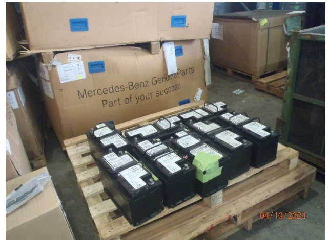
Picture 26 – CAA Lead Acid Batteries
