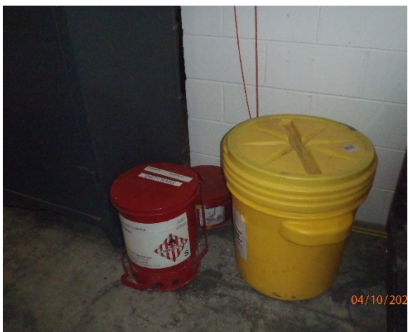
Picture 12 – Paint Shop Maintenance flip can SAA and spent solvent SAA
