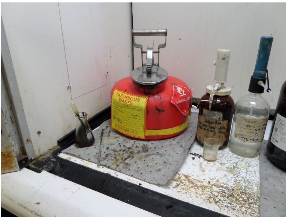
Photograph 5: Satellite Accumulation Container in Fume Hood
