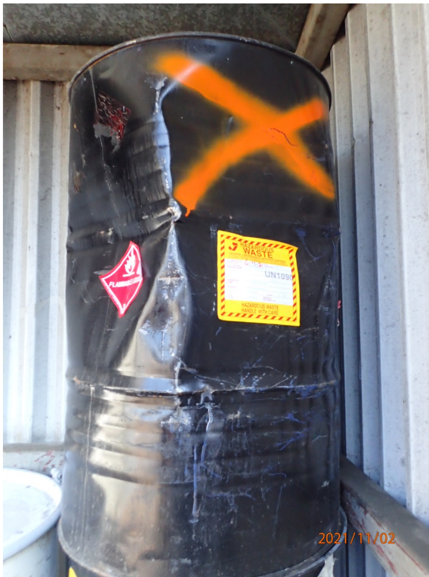
Photo 4: One (1) 55-gallon drum of waste acetone. The container was closed and labeled with the words “Hazardous Waste” and marked with an indication of hazard. The drum was dated 6/4/2021, which was over the 90-day accumulation storage limit.
