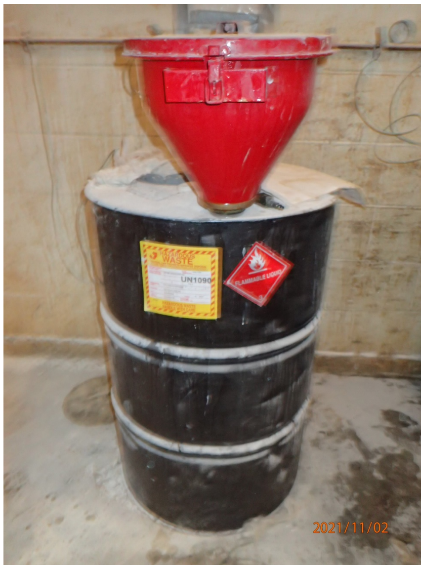
Photo 8: One (1) 55-gallon drum of waste acetone. The container was closed and labeled with the words "Hazardous Waste". The drum was not marked with the indication of hazard. This was corrected immediately onsite.
