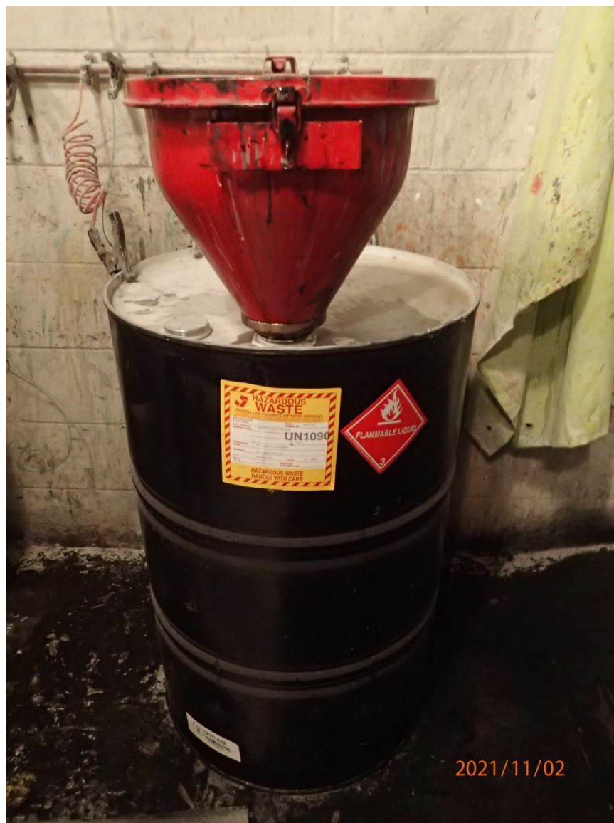
Photo 1: One (1) 55-gallon SAA hazardous waste drum containing waste acetone sludge. The container was closed and labeled with the words “Hazardous Waste”; however, the container was not marked with an indication of hazard. This was corrected immediately onsite.
