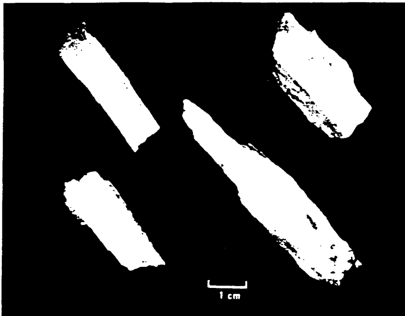
FIGURE 22. - Macrophotograph of spodumene ( \text{LiAlSi}_2\text{O}_6 ) showing prismatic shape (X 1).
