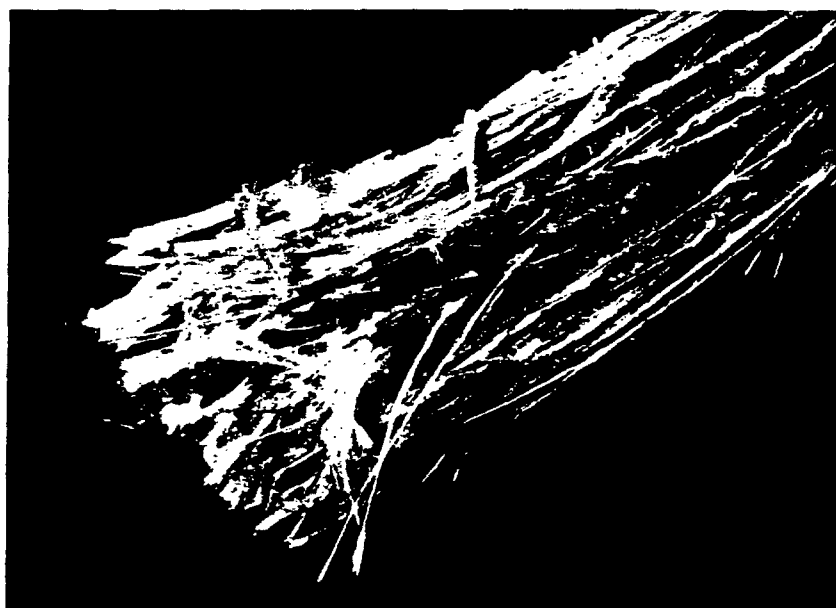
FIGURE 10. - Macrophotograph of anthophyllite asbestos (X 3).
