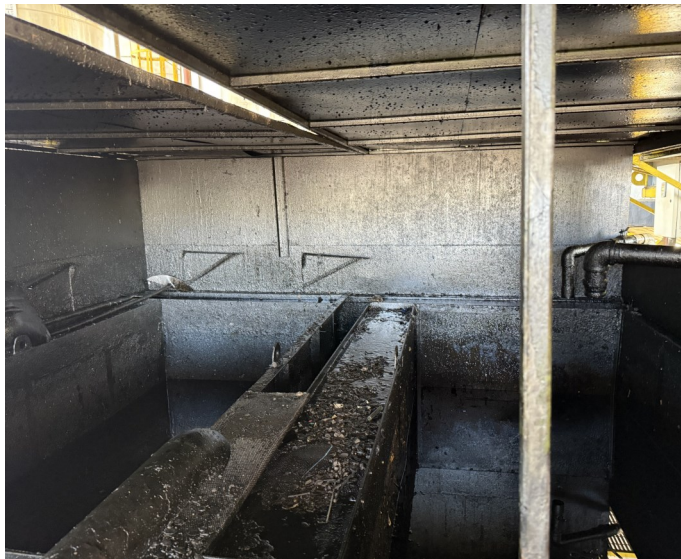
Picture 11 - OIL ENERGY SYSTEMS- At the Used Oil Filling Processing Area there were many detections of a release of used oil on the floor and potentially moving toward the environment outside of the secondary containment area and drain systems .
