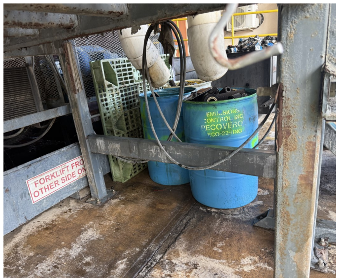
Picture 4 - OIL ENERGY SYSTEMS- At the Used Oil Filters Processing Area there were two (2) 55-gallon blue plastic drums with absorbent rags, paper, and used oil filters impacted with used oil which were on-going crushing processes and not labeled or marked clearly with the words, “Used Oil.”
