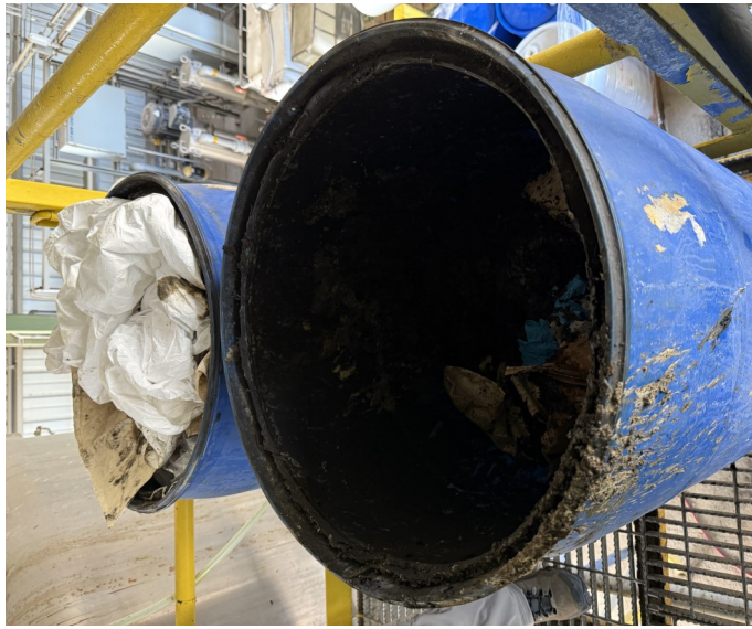
Picture 9 - OIL ENERGY SYSTEMS- At the Wastewater Treatment Plant there were two (2) 55-gallon blue plastic drums with absorbent rags, paper, and tyveks impacted with used oil not labeled or marked clearly with the words, “Used Oil,.”
