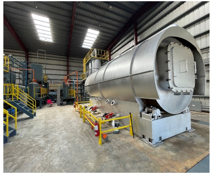
Picture 26 - OIL ENERGY SYSTEMS- At the Pyrolysis Plant there was one (1) aboveground reactor chamber connected to casing, oil tank, air blow, gas control, fuel condenser and air emission equipment among other auxiliary equipment running trial burns tests .
