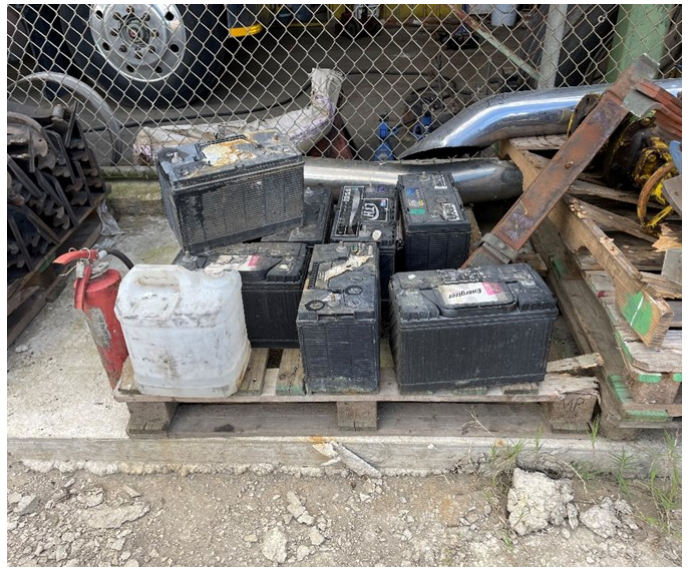
Picture 30 - OIL ENERGY SYSTEMS- At the Sidewalk Area there was eight (8) discarded spent acid-lead batteries and (1) discarded fire extinguisher along with brake pads, oily tools, and mechanical parts on a wood pallet in which no hazardous waste determination has been made on the discarded batteries and extinguisher ready for disposal.
