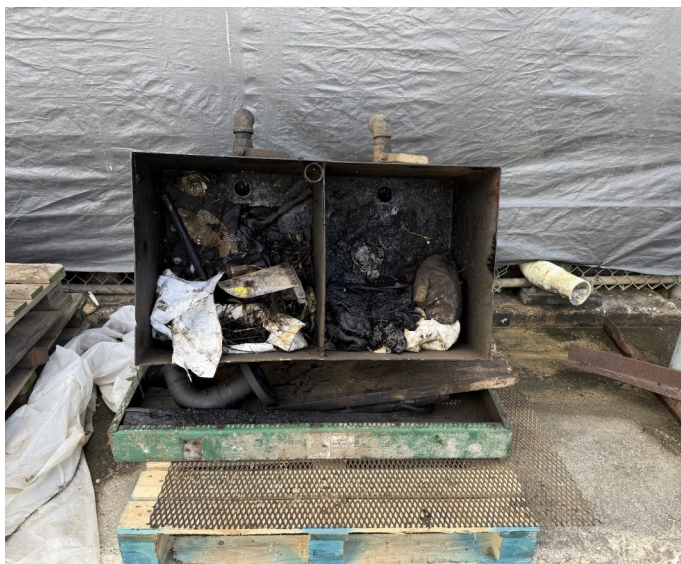
Picture 31-OIL ENERGY SYSTEMS- At the Sidewalk Area there was one (1) steel metal Part Washer abandoned with oily impacted rags, absorbent pads contaminated with used oil and fuel oil not labeled or marked clearly with the words, “Used Oil,.” nor hazardous waste determination of the content,
