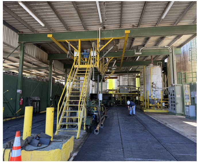
Picture 10 - OIL ENERGY SYSTEMS- EPA Inspector inspected the Used Oil Filling Processing Area. The process of receiving the used oils commenced with transferring the product into filling discharge tanks.
