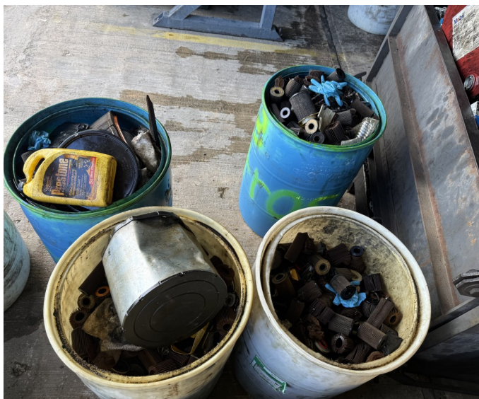
Picture 3 - OIL ENERGY SYSTEMS- At the Used Oil Filters Processing Area there were five (5) 55-gallon blue and yellow plastic drums with absorbent rags, gloves, used oil filters, and plastics impacted with used oil not labeled or marked clearly with the words, “Used Oil.”
