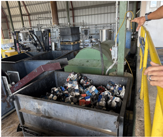
Picture 1 - OIL ENERGY SYSTEMS- At the Used Oil Filters Processing Area there were two (2) 3-cubic yard (cy) metal containers with compacted filters and residual used oil liquids not labeled or marked clearly with the words, “Used Oil.”
