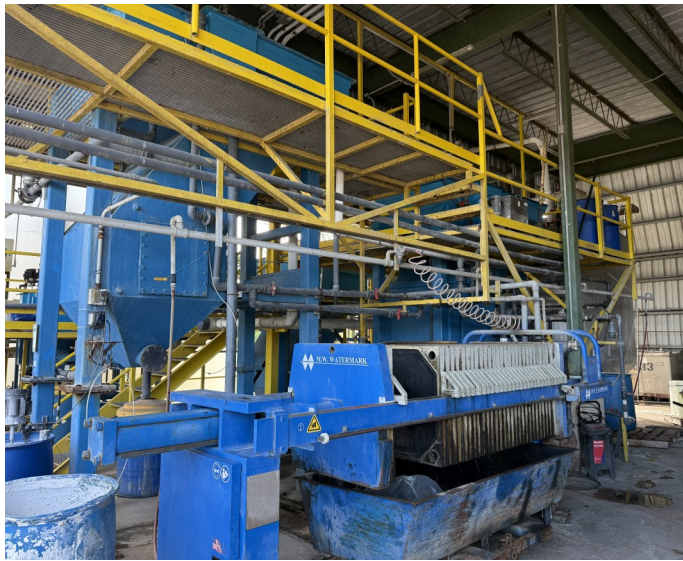
Picture 7 - OIL ENERGY SYSTEMS- At the Wastewater Treatment Plant the process consists of separating remnant oil and sediments from the contact water obtained from the decantation tank.
