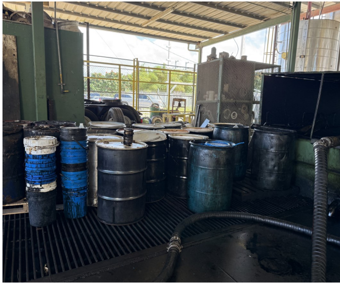
Picture 13- OIL ENERGY SYSTEMS — At the Used Oil Filling Processing Area there were twenty-four (24) 55-gallon blue/black plastic/steel drums with used oils, some had absorbent rags impacted with used oil, others were empty sitting on releases of used oil on the floor that were not labeled or marked clearly with the words, “Used Oil,.”
