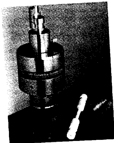
MODEL 686.03 CERAMIC TENSILE GRIP — Only 18 lbs. per grip; this device features an easy-to-use two-piece collar, a patented floating piston for minimal bending strain and eight times fewer moving parts than other designs.
