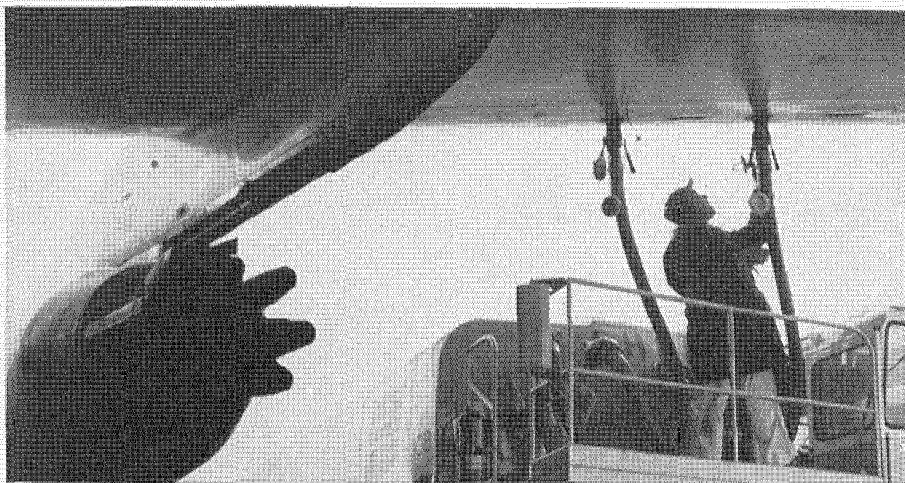
Refueling in 1930's was by hand pump from back of truck, left. Underwing loading, right, came later, greatly reduced costly on-ground time.
