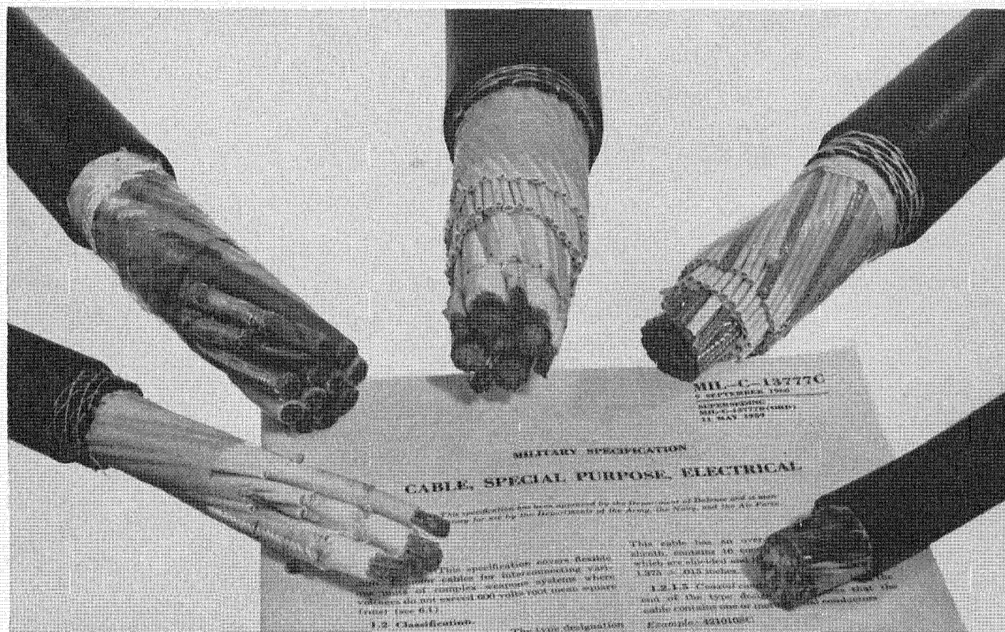
Complex missile cable may have nylon-armored polyethylene insulation on conductors; a binder of "Mylar"; an outer jacket of neoprene.
