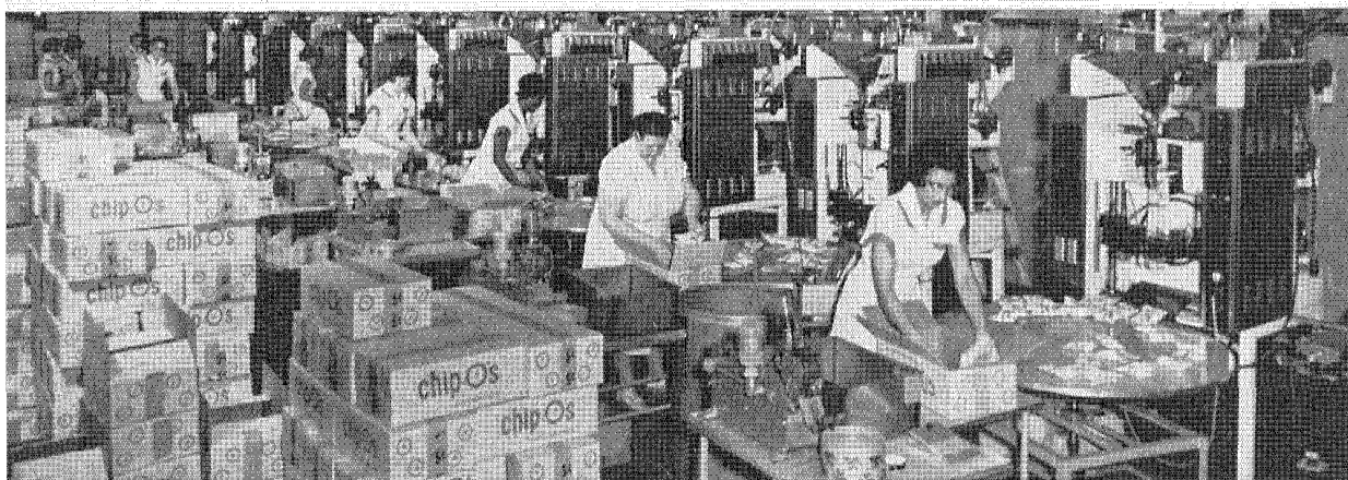
Nine form-and-fill packaging machines turn out 18,000 cellophane bags of chip-O's per hour.
