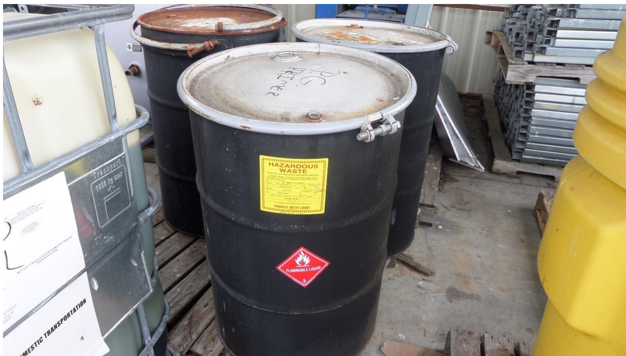
Photograph 10: View of PG Primer hazardous waste container located in the CAA adjacent to the Maintenance Shop Container. Containers were labeled during the inspection.
