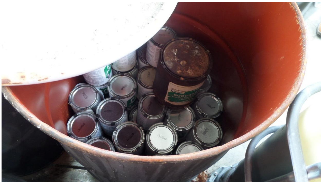
Photograph 9: View of hazardous waste, PG Primer, located in the central accumulation storage area adjacent to the Maintenance Shop Containers. The containers were unlabeled at the time of the inspection.
