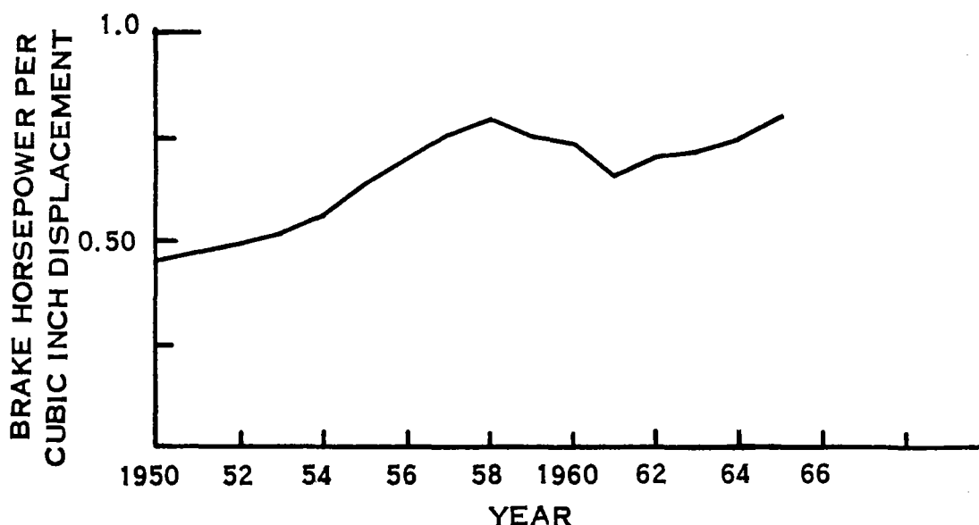
Figure 4 — Trend in passenger car engine brake horsepower per cubic inch of engine displacement.
