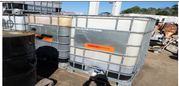
Photo-23 Unlabeled Used Oil Tote
