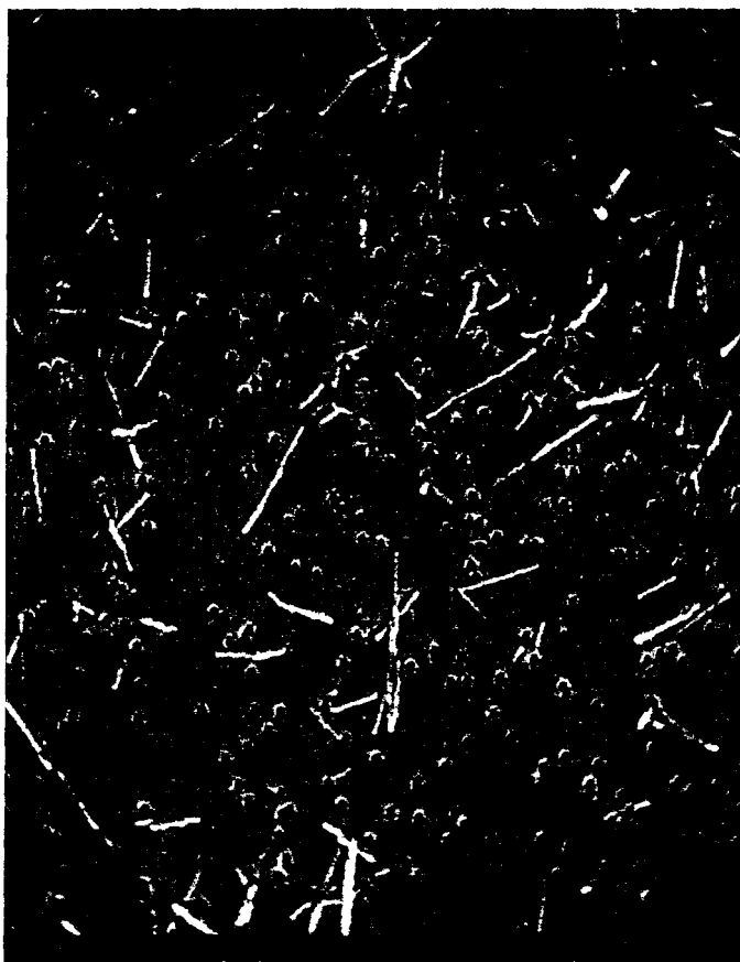
FIGURE 14 CHRYSOTILE ASBESTOS FIBERS IN FILTRATE FROM 0.8 \mu M NUCLEPORE MEMBRANE-CHALLENGED WITH 1.29x10 11 FIBERS, 10,000 X SEM
