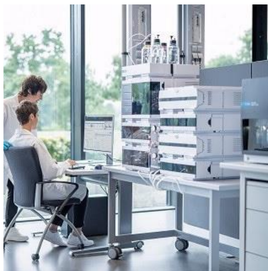
Figure 1: A typical high-performance LC/MS system for laboratory analysis. Samples and solvents are drawn from the top of the instrument, degassed, pressurized, and separated prior to analysis within the Mass Spectrometer.
