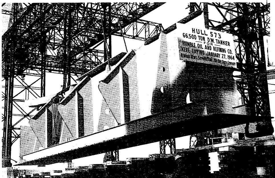
Freshly coated with Rust-Ban 191, first bottom section assembly for Humble's 66,700-dwt. supertanker is lowered to keel blocks at Newport News.
