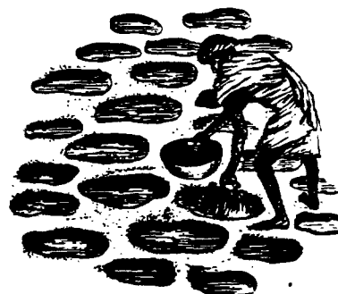
In Asia salt is laboriously obtained by evaporation. A worker is collecting the dry salt crust from each basin
