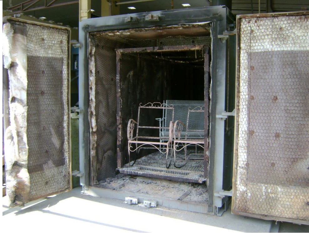
Incinerator with metal chairs inside. Used for removing coatings from parts.
