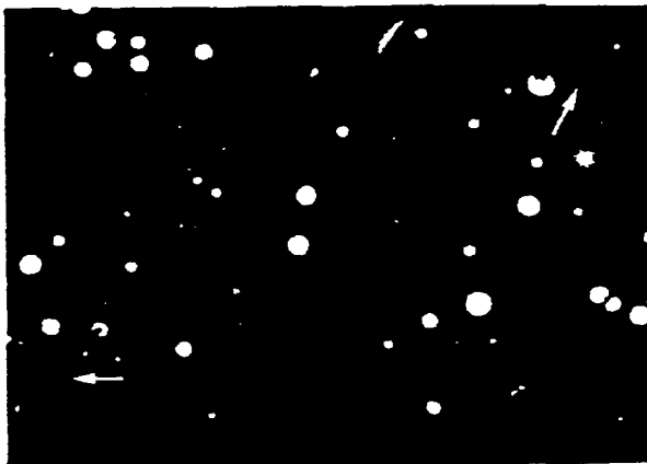
Fig. 5. A transmission electron microscope photograph of small dust particles from the ceramic fibre cloud; magnification, 6000x
