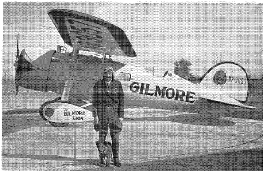
The glass-like Duco finish on the plane, "Gilmore Lion," increases air speed ten miles per hour, according to the engineers.
