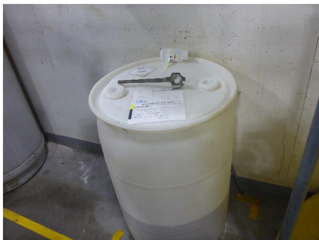
Photo 14: One 55-gallon container in the second SAA in the Plating Area. The container was labeled as UN1935 hazardous waste cyanide solutions (potassium silver cyanide); it was marked with EPA hazardous waste numbers D003 and F007; and it was identified with a DOT hazard sticker indicating that the contents are toxic.
