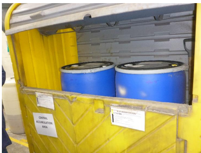
Photo 15: CAA for accumulating and storing used wipes, filters, PPE and other solids contaminated with plating bath solutions. The clam shell held two 55-gallon containers: one labeled as Ag filters, identified as toxic, and dated February 20, 2024, and one labeled as gold filters, identified as toxic, and dated February 20, 2024. Neither container was labeled with the words “hazardous waste,” but the clam shell was labeled as “UN 1588 hazardous waste cyanides (potassium gold cyanide) D003, F007” and “UN 1588 hazardous waste cyanides (potassium gold cyanide) D003, F007.”
