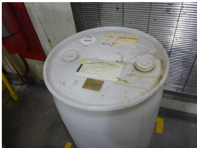
Photo 13: One 55-gallon container observed in the first SAA in the Plating Area. The container was labeled as UN1935 hazardous waste cyanide solutions (potassium gold cyanide); it was marked with EPA hazardous waste numbers D003 and F007; and it was identified with a DOT hazard sticker indicating that the contents are toxic.
