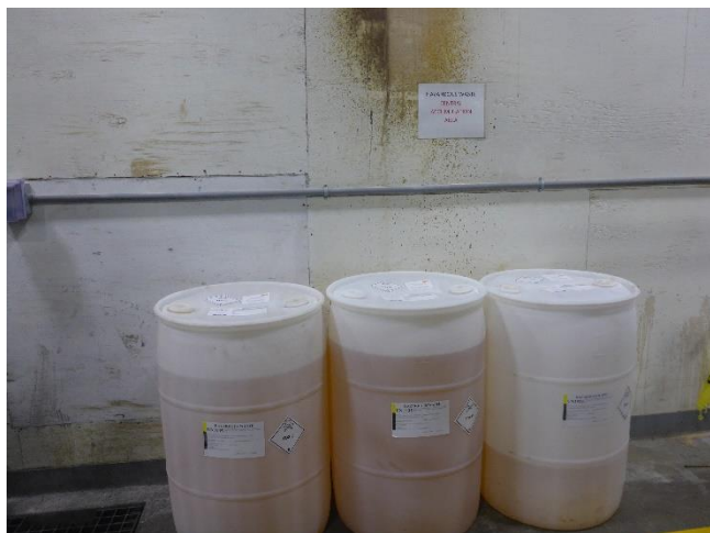
Photo 16: CAA in the Plating Area for accumulating and storing old process material that will be sent off-site for reclamation.
