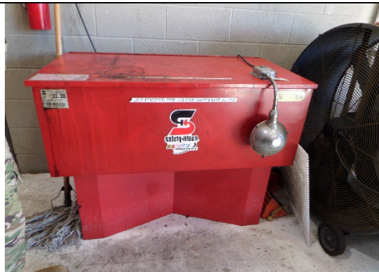
Photo-11 Unlabeled Safety-Kleen Parts Washer Unit
