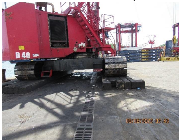
IMG 489 -Crain staged on dock platform for loading and unloading cargo. IMG 490 -View of the crain track system along the active dock where loading and unloading occurs. Drain collects stormwater runoff, oil and grease leaks and spills installed in place. View of drain along the entire dock bulkhead.
