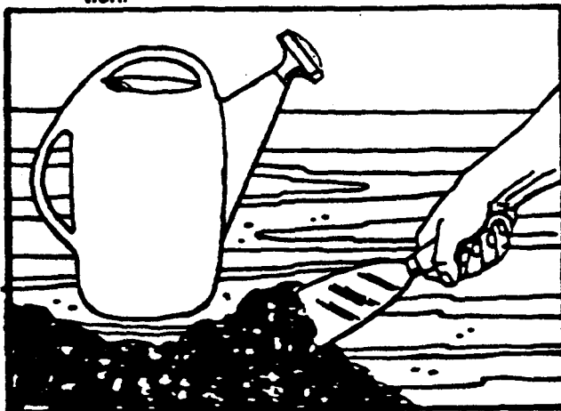
Sketch 12. After wetting felt, use stiff-bladed scraper to remove.
