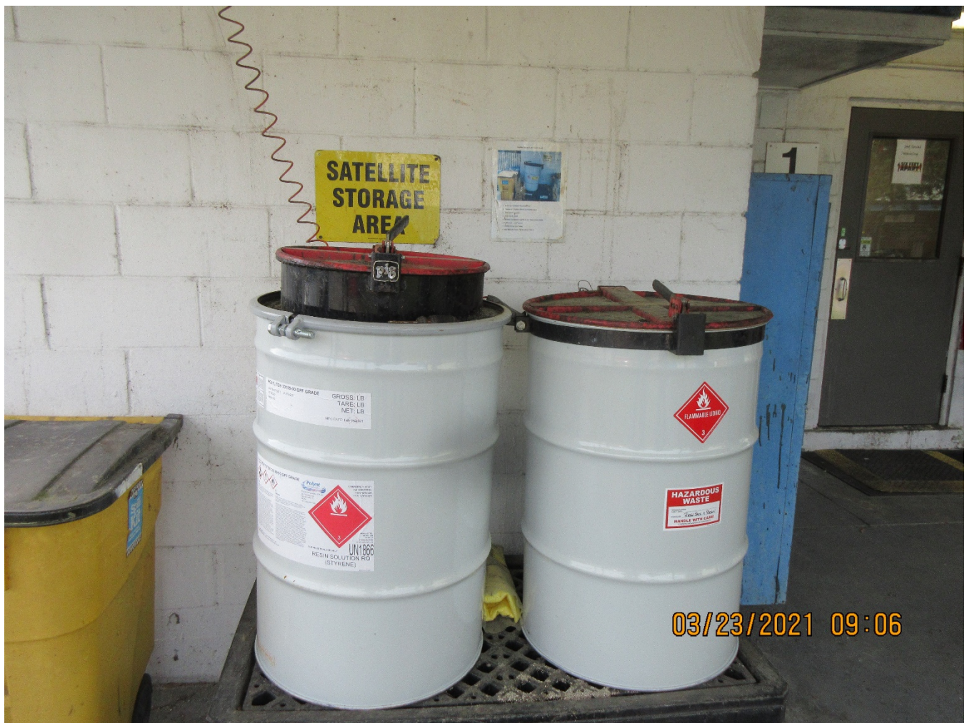
Photo 1 – Hazardous waste drum outside of the Quality Control Lab receiving resin jars used for holding samples
