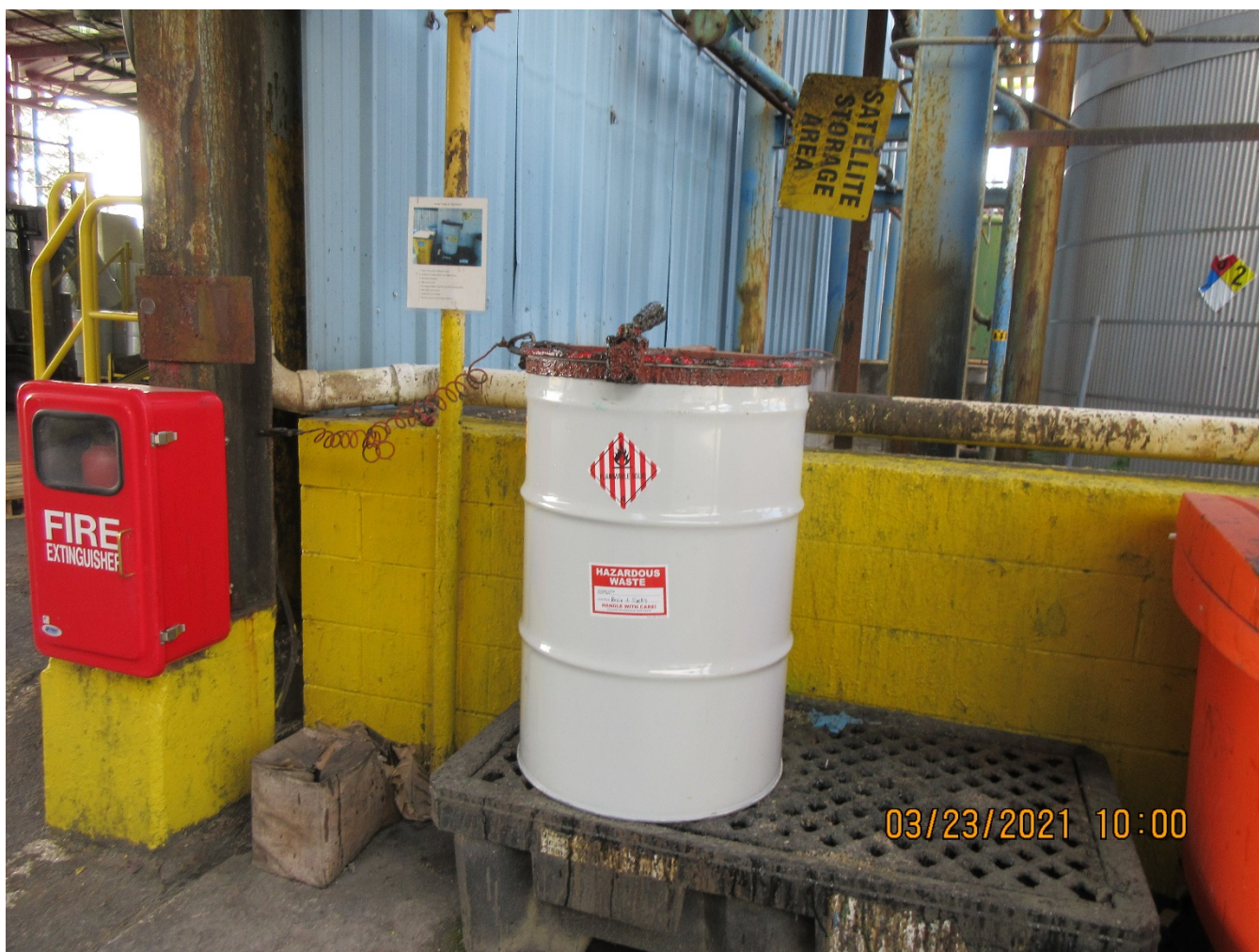
Photo 9 – Hazardous waste accumulation container for socks in the truck offloading area.
