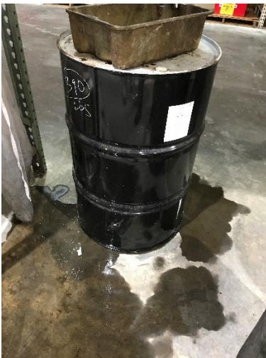
Photo-18 D001 Waste Spill
