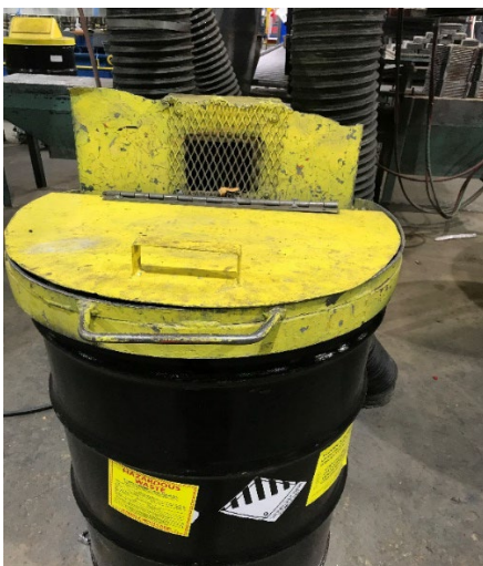
Photo-27 Burn Box Open SAA Container
