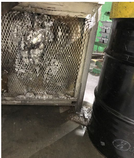
Photo-14 D008 Waste Dross Waste on the Floor
