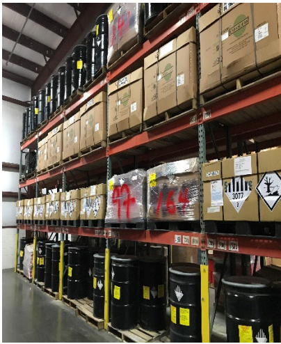
Photo-23 CAA Inadequate Aisle Space and Class 9 Hazard Indication
