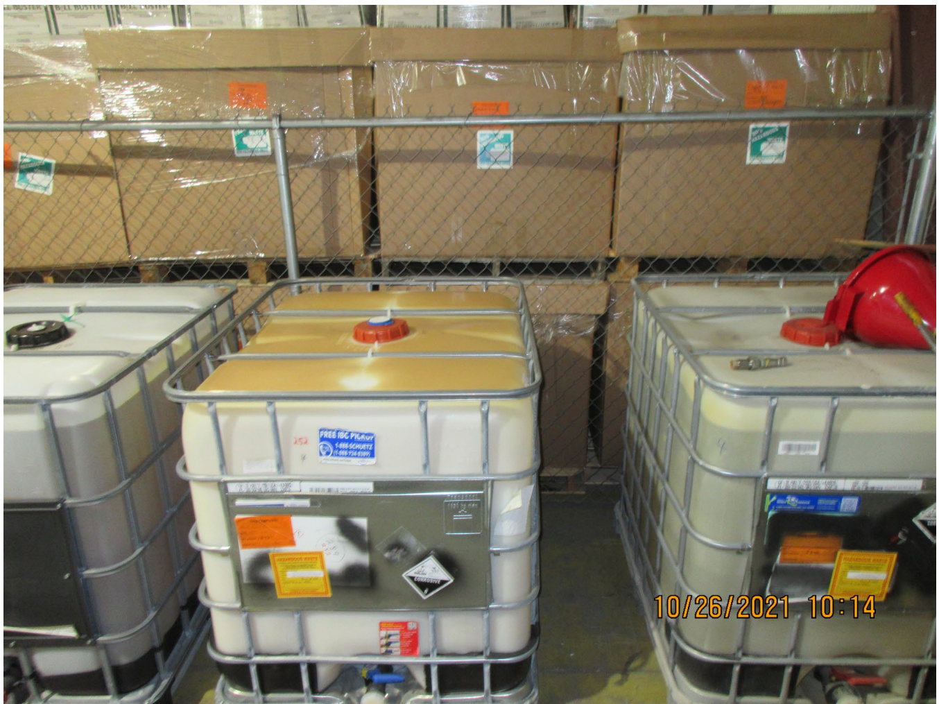
Photo 6 – Totes of D002 corrosive hazardous waste from the Ethephon area located in the facility's 90-day accumulation area within Warehouse One.
