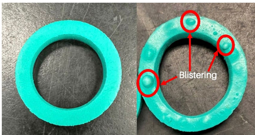
Figure 3. Before and after pictures of an elastomer that underwent rapid gas decompression
