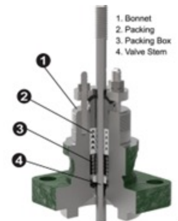
Figure 18. PTFE valve packing example
