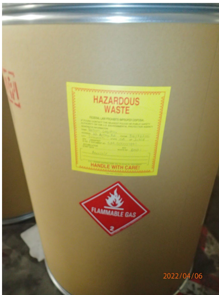
Photo 7: One (1) 35-gallon closed drum of waste aerosol cans. The drum was labeled with the words "Hazardous Waste" but not marked with an indication of hazard.
