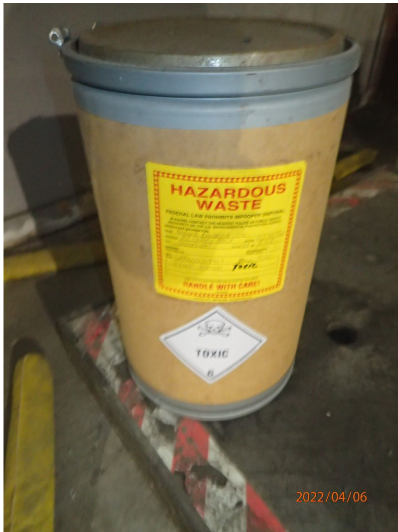
Photo 6: One (1) 5-gallon closed container of silver nitrate. Initially not marked with an indication of hazard. Corrected during the inspection.
