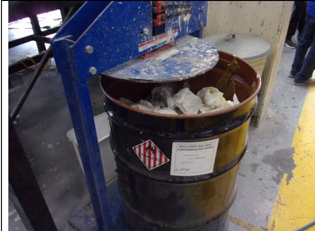
Figure 17: 12:26 PM Building G Picture two of two opened 55-gallon SAA containers observed.
