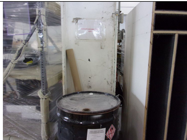
Figure 15: 12:23 PM Building G One opened 55-gallon SAA containers observed.
