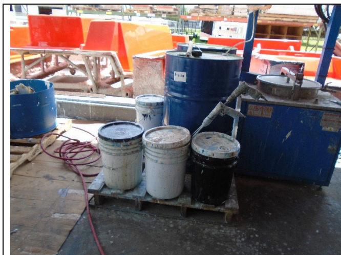
Figure 33: 10:56 AM Distill/Kick-off Area Four (4) 5-gallon containers adjacent to the kick-off machine with no label or indication of the hazards of the contents. Photo provided by FDEP.
