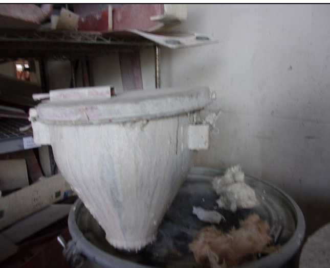
Figure 24: 12:58 PM Commodore Building Lamination One of two 55-gallon containers observed with funnel unsecured.
