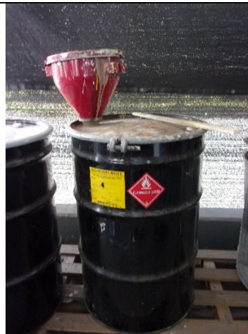
Figure 8: 11:39 AM 90-Day Storage Area One 55-gallon container of hazardous waste adhesive observed.
