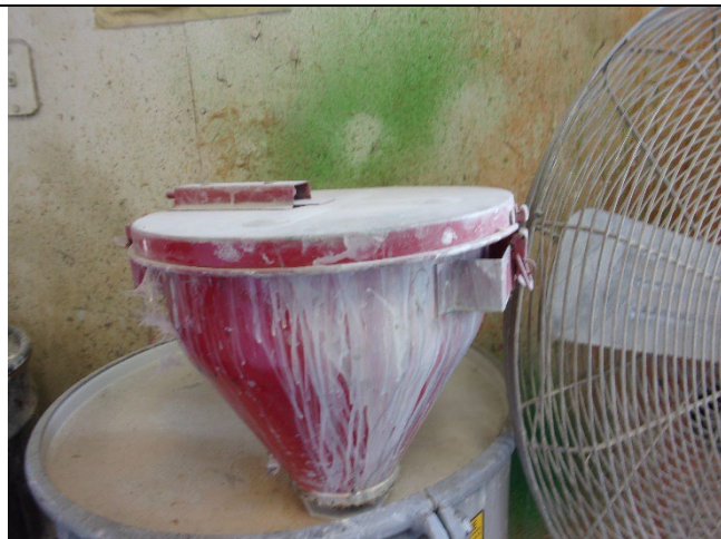
Figure 14: 12:19 PM Building D CAA One of the two (2) 55-gallon container with unsecured funnel observed.
