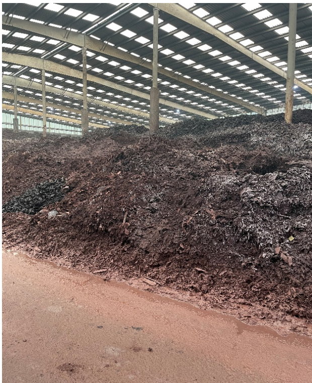
Photo 1: Lead Bearing battery pieces from Hammer Mill System.
