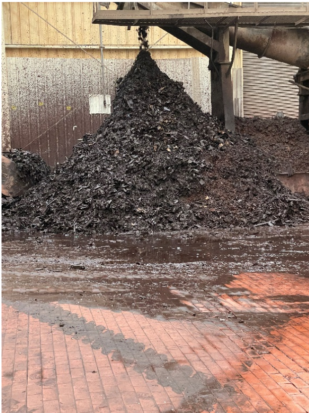
Photo 1: Lead Bearing battery pieces from Hammer Mill System.
