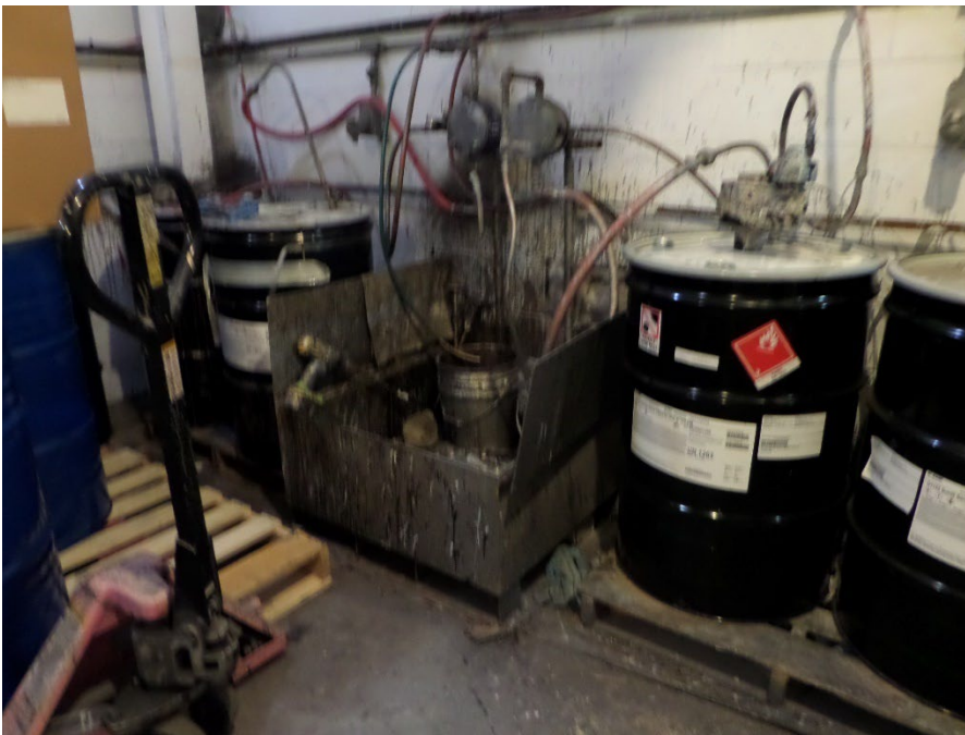
Photograph 14: Second Photograph of Open HW Containers in the Paint Mix Room Containers are not Labeled as HW Containers and are Missing the Hazard Indication Label.
