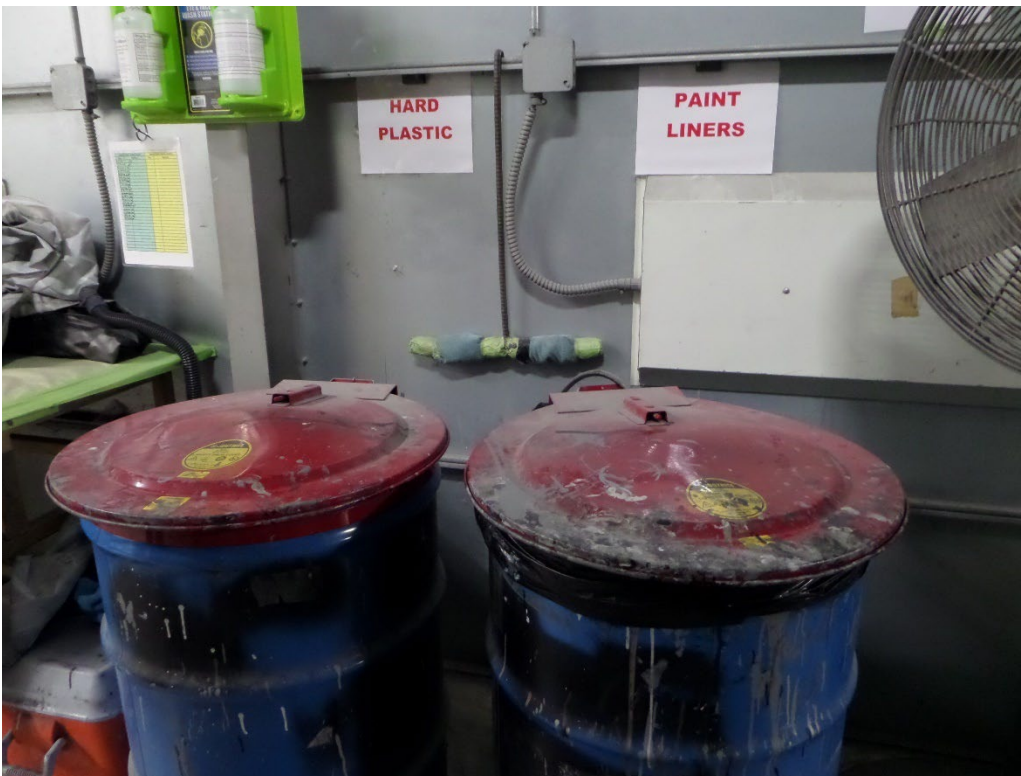
Photograph 10: SAA HW Drums Without HW and Without Hazard Labeling
