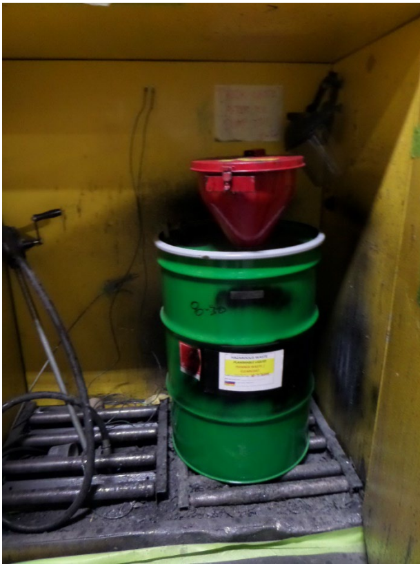
Photograph 11: SAA HW Drum With Partially Obscured Hazard Label
