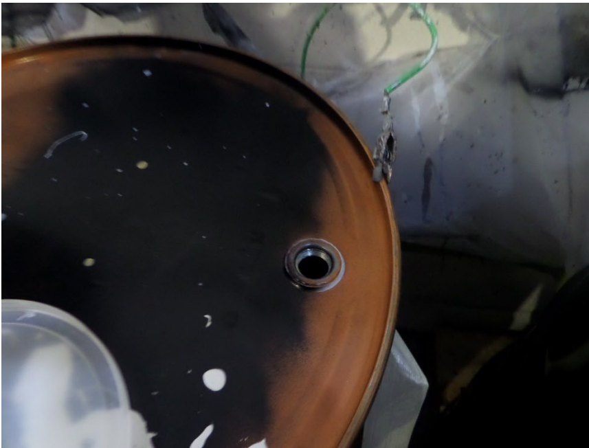
Photograph 15: Open SAA HW 55-Gallon Drum in Paint Mix Room
