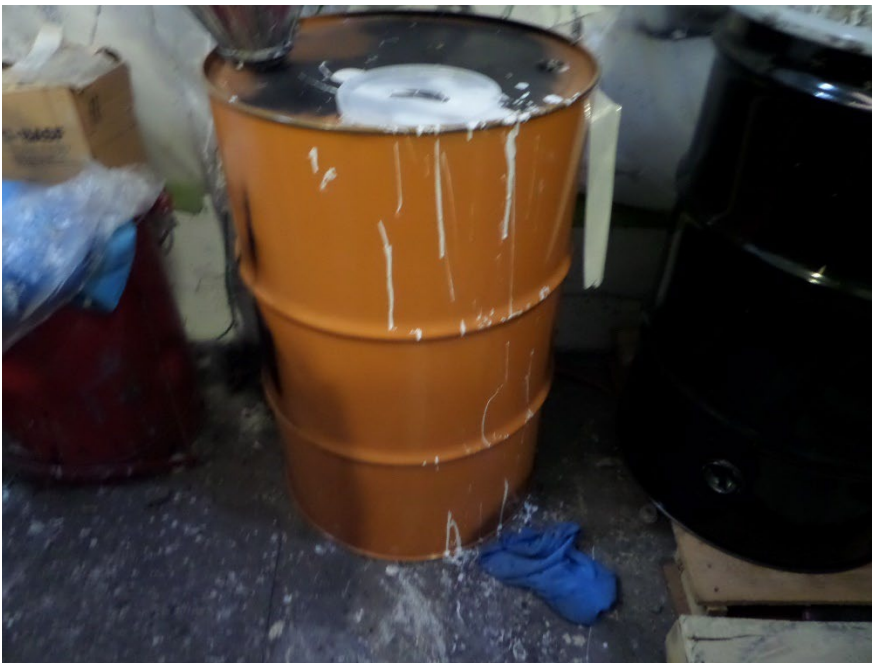
Photograph 16: Open HW SAA 55-Gallon Drum That is Not Labeled as Hazardous Waste and is Missing the Hazard Marking
