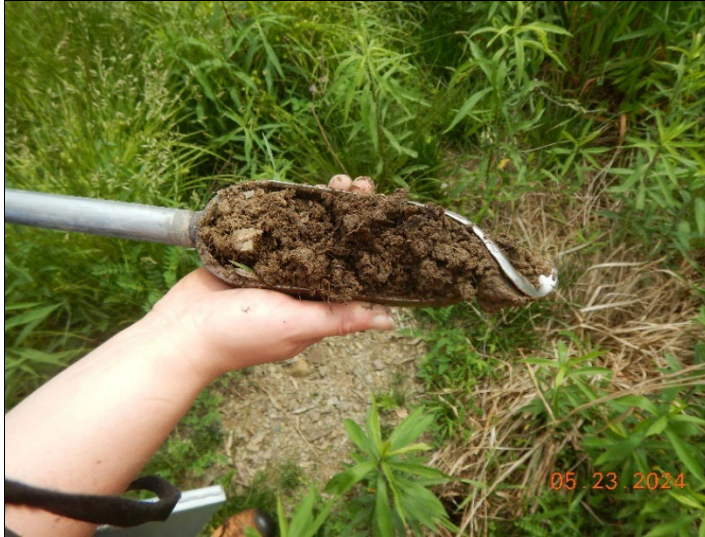
Terrace at Maplewood Date: 23 May 2024 Photo ID: DSCN5391.JPG Photo taken by: Katelyn Almeter Notes: Soil boring with fill material.
