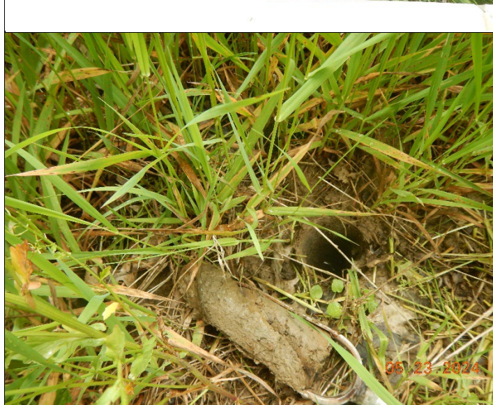
Terrace at Maplewood Date: 23 May 2024 Photo ID: DSCN5387.JPG Photo taken by: Katelyn Almeter Notes: Soil boring showing a saturated, undisturbed soil profile. Water table present in soil pit.
