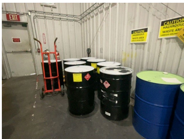
Photo 12: 90-Day CAA. All containers were closed, labeled, marked with an indication of the hazard of the contents, and dated.
