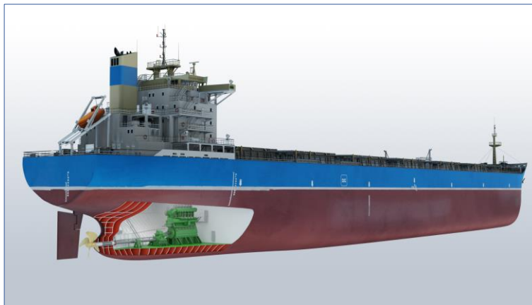
Figure 1a: Propulsion system of a vessel. Courtesy of AEGIR Marine BV.
