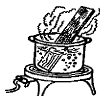
Immersion in boiling water for 15 hours produces no more than moderate whitening and recovery is complete in 1/4 hour.
